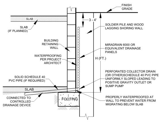
**Shoring Retaining Wall Drainage Detail**
