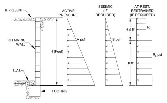
**Retaining Wall Loading Diagram**
