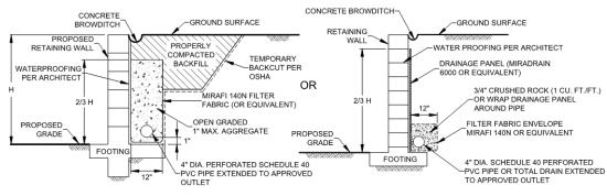
**Typical Retaining Wall Drainage Detail**
