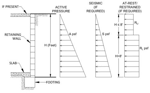
**Retaining Wall Loading Diagram**
