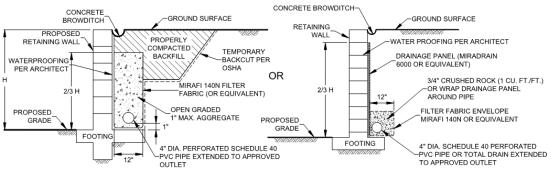
**Typical Retaining Wall Drainage Detail**
