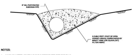
1.....8-INCH DIAMETER, SCHEDULE 80 PVC PERFORATED PIPE FOR FILLS IN EXCESS OF 100-FEET IN DEPTH OR A PIPE LENGTH OF LONGER THAN 500 FEET.
