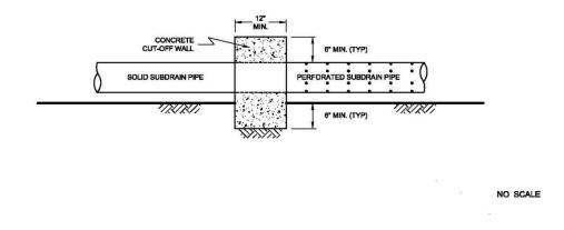
7.6 Subdrains that discharge into a natural drainage course or open space area should be provided with a permanent headwall structure.
