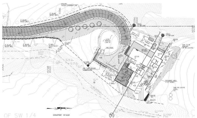
Figure 2. Grading Plan for the proposed project with 25-foot setbacks from the riparian woodland.
