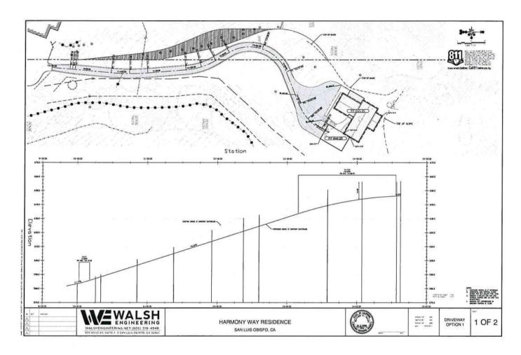
Figure 6. The design, location, and topography of the driveway and home site on Harmony Way. The owner will provide a larger, more readable version of this illustration.
