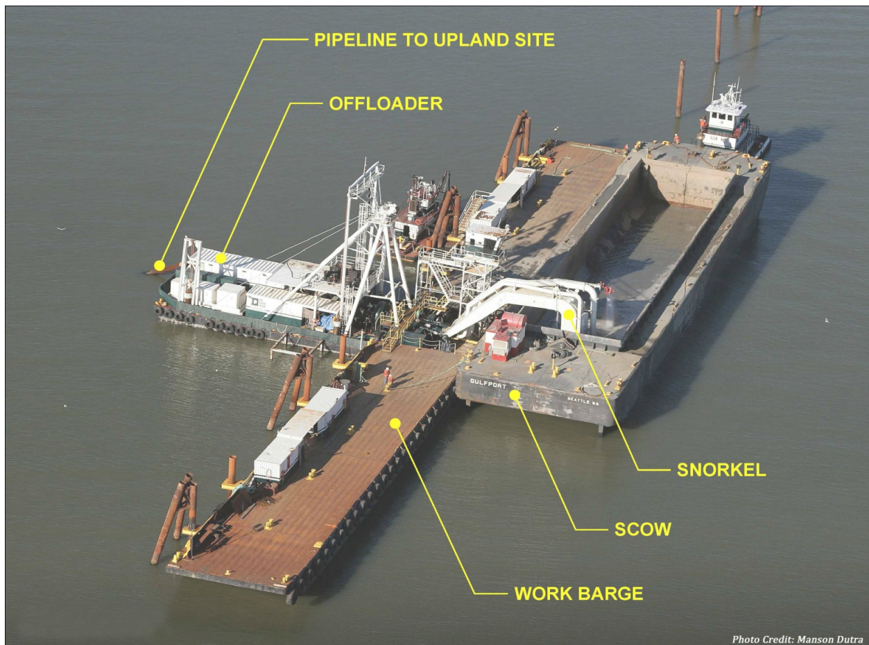
Figure 7 – Offloader Liberty Unloading Scow.
