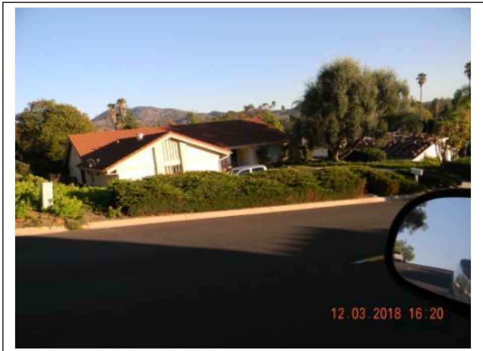
Photo 7: Another view of a home on the east side of Saint Andrews Drive with a highly flammable juniper hedge. This juniper, when it burns will produce enough prolonged radiant heat to ignite the structure and compromises the safety of escaping evacuees and arriving first responders using Saint Andrews Drive (Photo by Mike Rogers).
