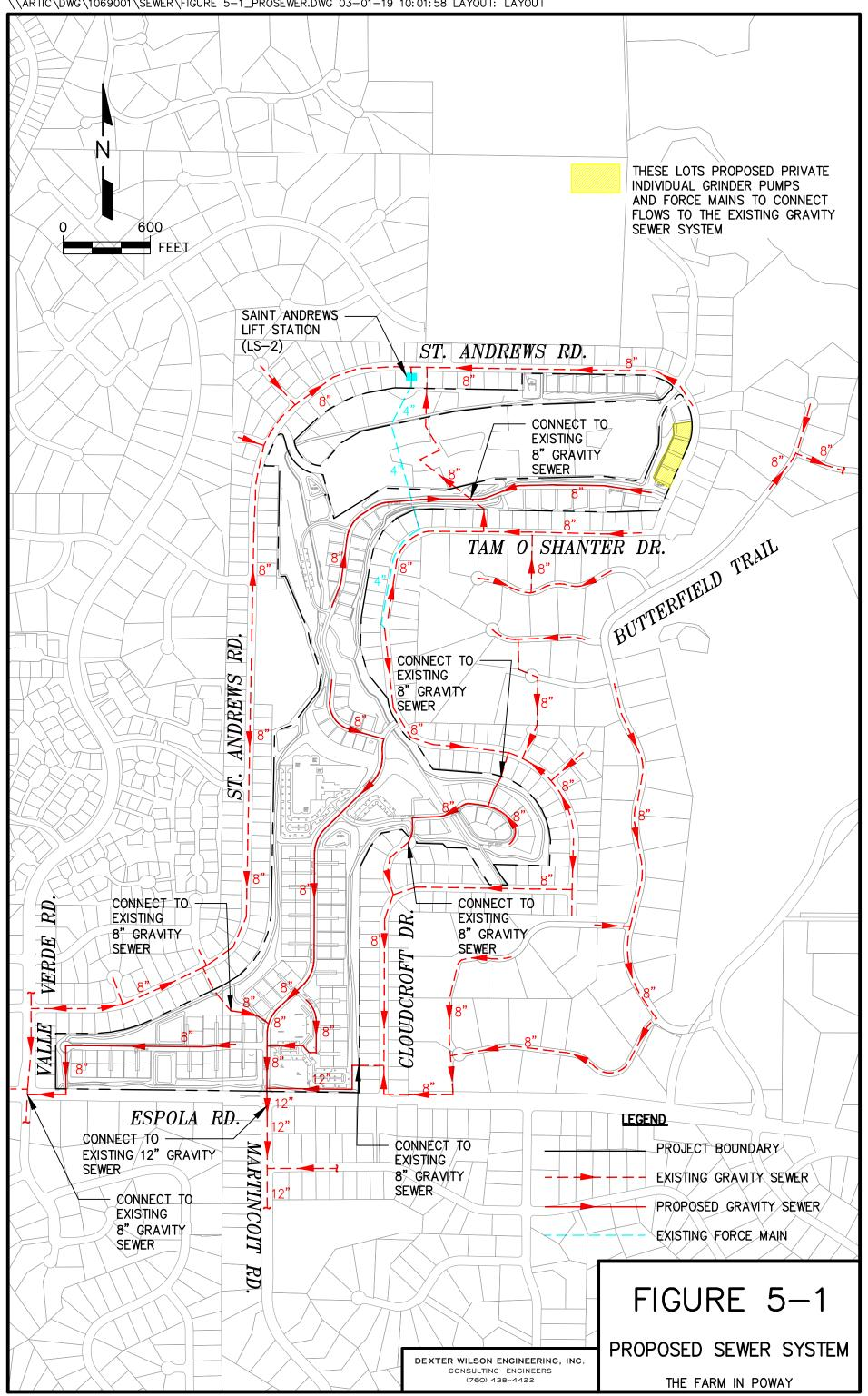
There are 34 lots in the southwest corner of the project that propose to convey flow westerly and connect to an existing 8-inch gravity sewer line at the intersection of Espola Road and Valle Verde Road. This gravity sewer line conveys flow south in Valle Verde Road.
