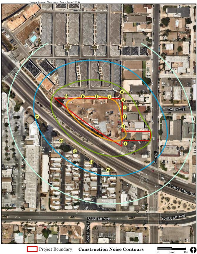
Project Boundary **Construction Noise Contours** Modeled Receivers 60 dB(A) Leq  $\bigcirc$ • 65 dB(A) Leq • 70 dB(A) Leq RECON M:\JOBS5\9010\common\_gis\fig7\_env.mxd 9/6/2018 sab 75 dB(A) Leq
