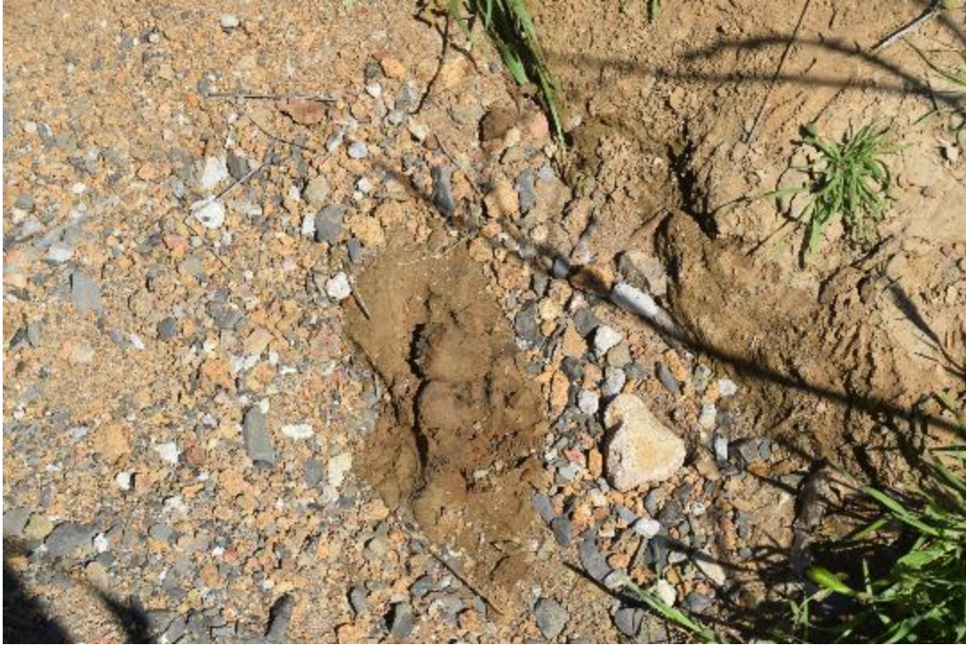
Photo 11. Evidence of surface saturation near the soil test pit in Feature 3. Soil expressed moisture when squeezed and was malleable.
