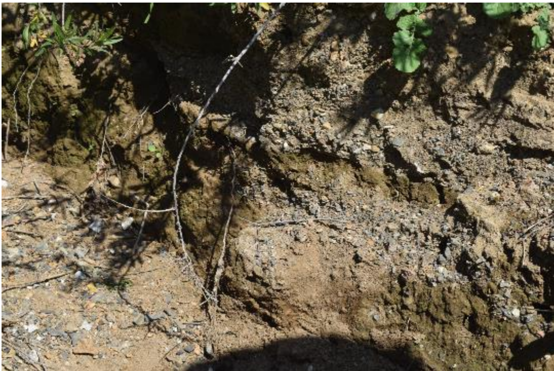
Photo 12. Additional evidence of surface saturation near the soil test pit in Feature 3. The dark bands are saturated or near saturated soil.
