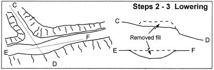
2. Remove any existing drainage structures including culverts and Humboldt logs.
