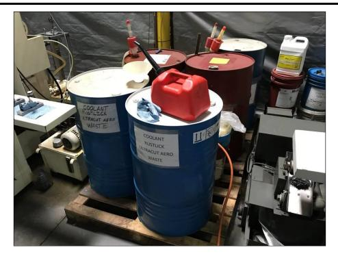
Photograph No. 11 View of properly sealed and labeled coolant waste and waste-oil located in the machining area of the warehouse.
