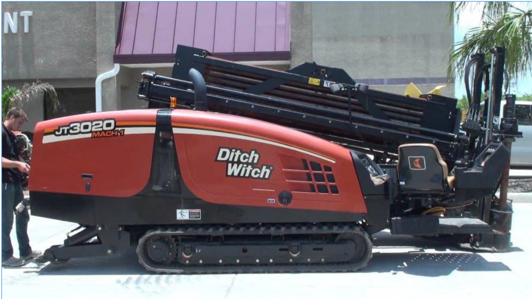
Photo 2.1 Typical directional boring machine used for fiber optic cable installation
