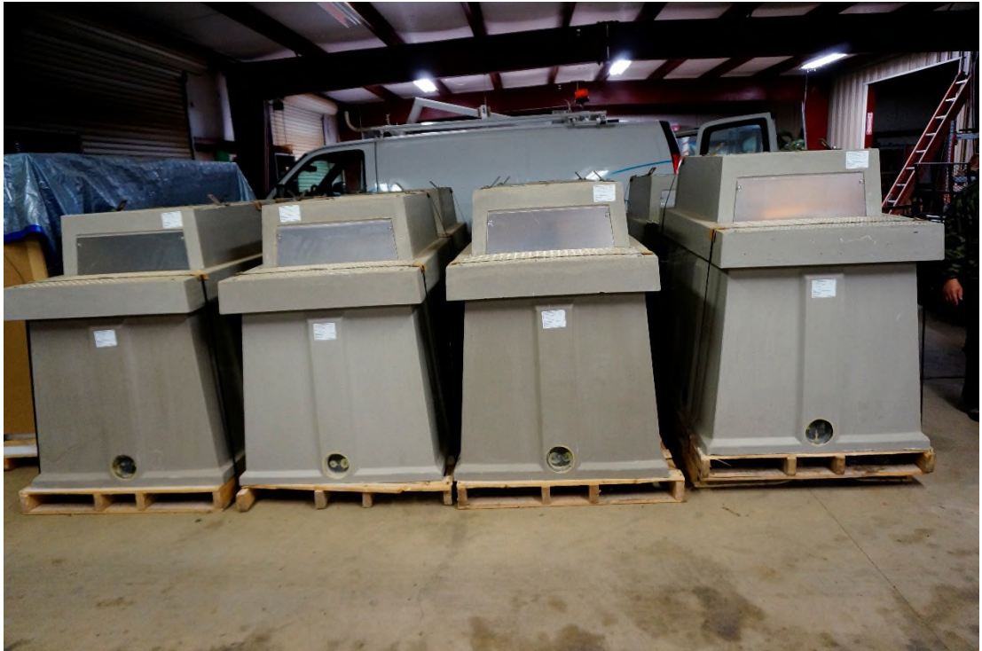
Photo 3. Examples of the new underground concrete and epoxy vaults (handholes) that would be installed at each of the seven new DLC sites and at any of the six existing DLC where renovation activities would include replacement of the existing underground vaults. The 'cap' of the vault, on which the small platform with a metal plate on the side is located, is the portion of the vault that would be aboveground. The remainder of the vault would be underground.
