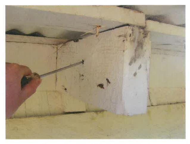
Figure 42. Testing by probes conducted during the field investigation. View of a rafter exposed to the exterior.
