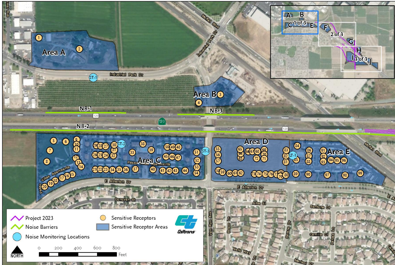
Figure 1. Analysis Areas, Noise Monitoring Positions, and Location of Evaluated Noise Barrier (2023)
