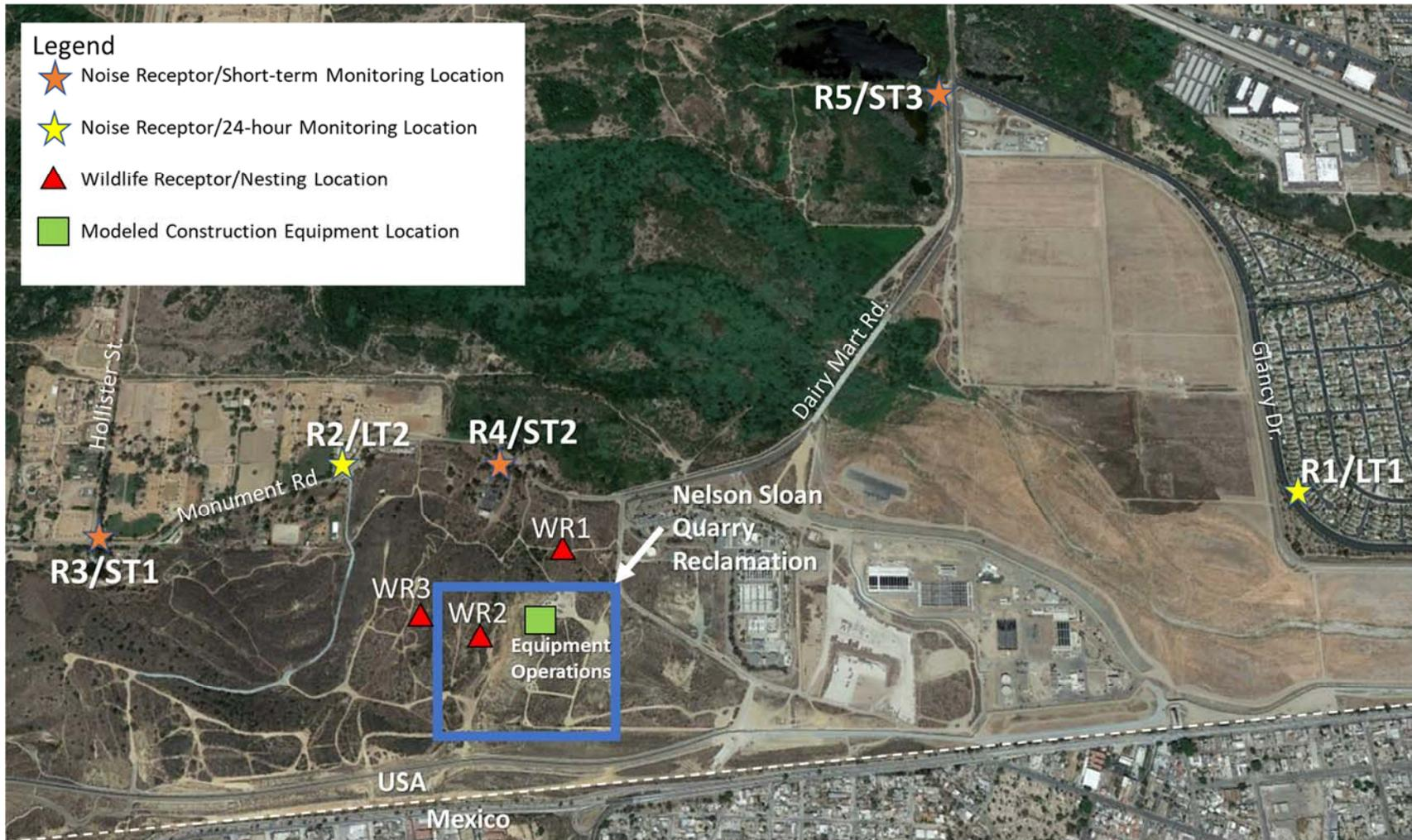
*\*For noise modeling purposes, the construction equipment location was chosen for proximity to the wildlife receptors.*
