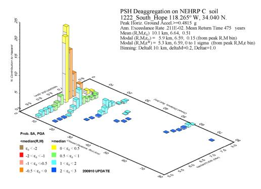
GMT 2016 Mar 18 17:43:36 Distance (R), magnitude (M), epsilon (E0,E) deaggregation for a site on soil with average vs= 440, m/s top 30 m, USGS CGHT PSHA2008 UPDATE Bins with it 0.05% contrib. omitte
