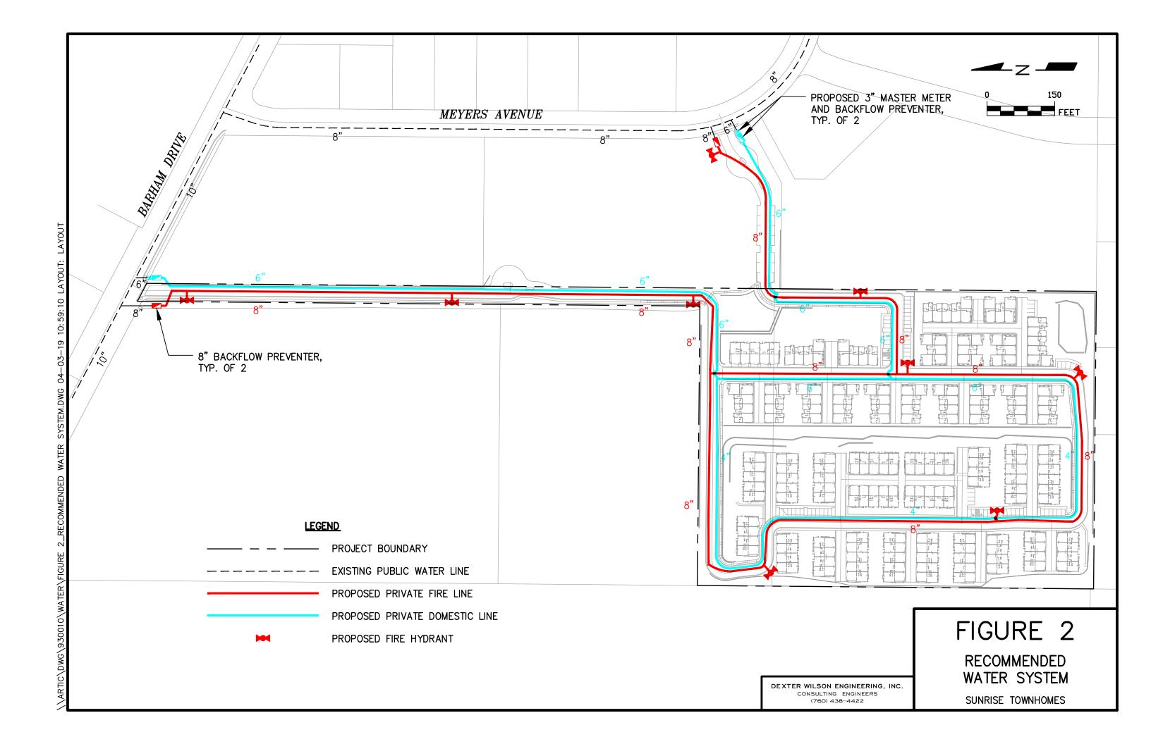
Meter Sizing. The meter size for the project was determined based on the total number of fixture units that will be served by the meter. Based on a peak water demand of 591 gpm, two 3-inch meters are recommended. The capacity of a 3-inch meter can range based on manufacturer and meter type, but capacities of 320 gpm to 400 gpm for a 3-inch meter are typical. Thus, two 3-inch meters have adequate capacity to meet the peak demands of the project.
