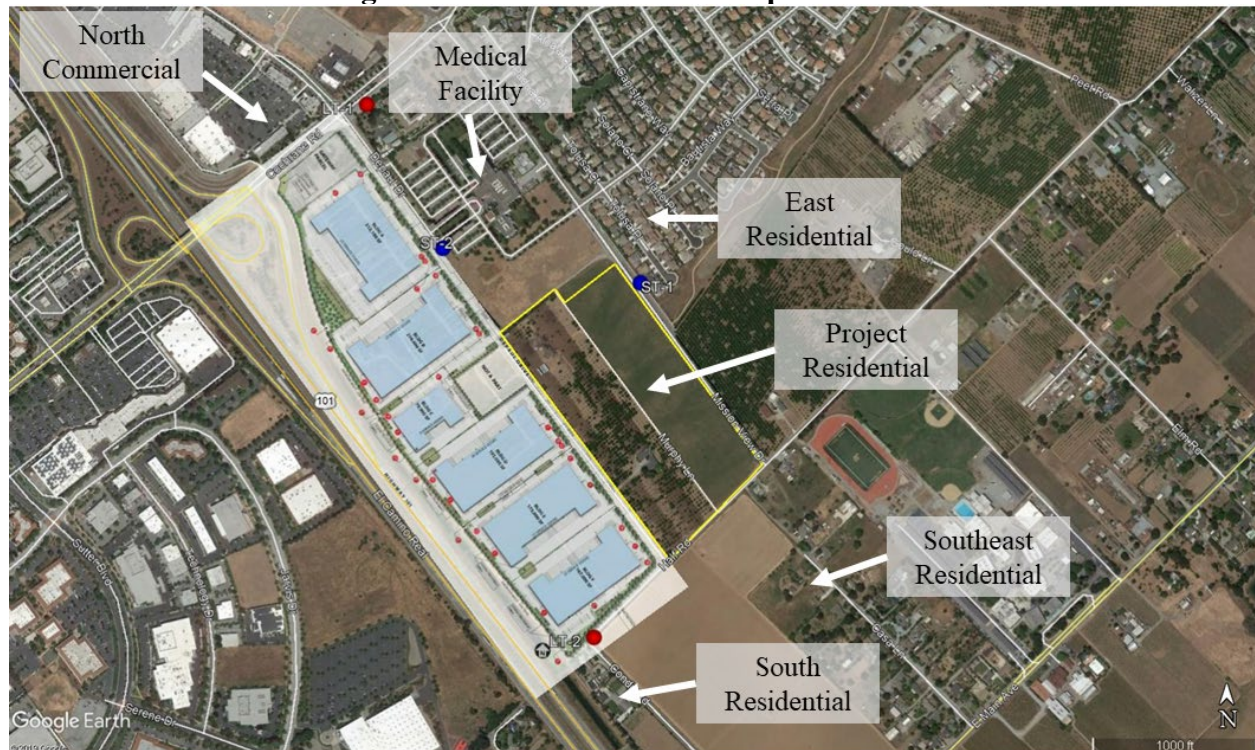
FIGURE 8 Surrounding Land Uses Evaluated for Exposure to Construction Noise Levels
