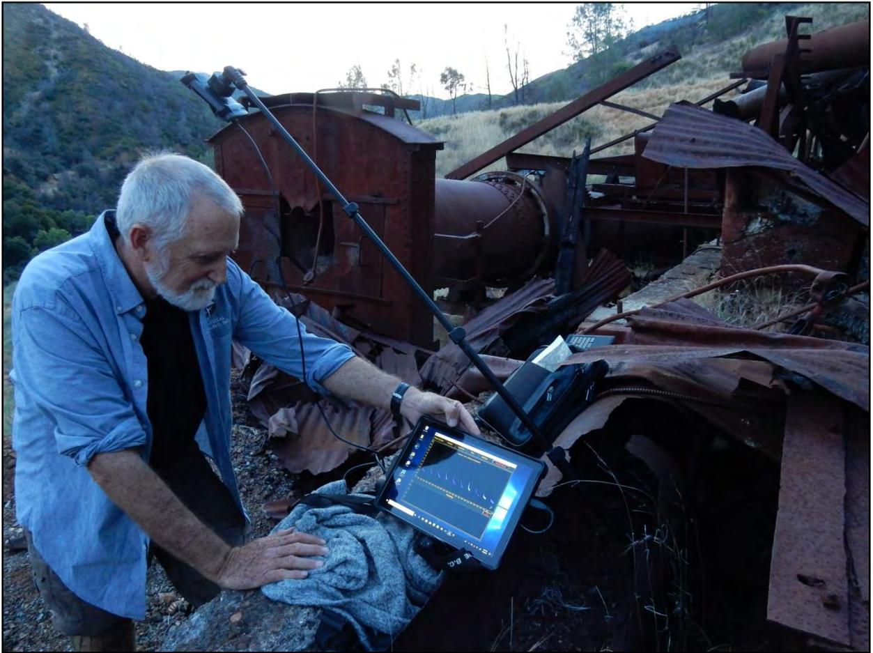
Figure 4. Acoustic monitoring equipment showing the ultrasonic microphone on the pole and a Sonobat Live display of a bat call on the laptop. (Photo by B. Keeley)
