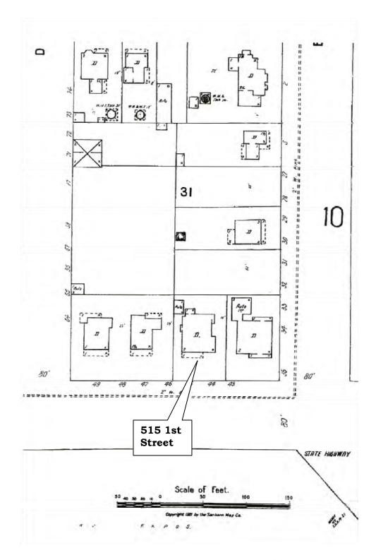
**FIGURE 24:** Sanborn Fire Insurance Map, Davis, California, 1921. Note that the auto garage in the rear no longer exists. The half porch is also illustrated in the Sanborn Fire Insurance Map before it was removed and expanded to form a full front porch or veranda.
