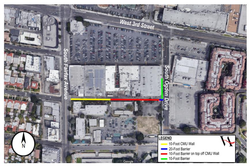
Figure IV.F-4 Proposed Construction Nose Barrier Diagram (Revised)
