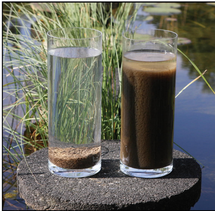
Figure 5-6 – Comparing Settling Characteristics with Aerobic Granular Sludge on left versus Conventional Activated Sludge on right (source: Aqua Aerobic Systems, Inc.)
