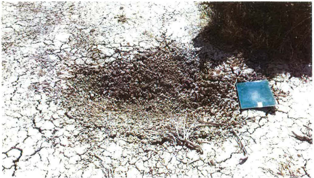
Example of a sinkhole within site – clipboard for size representation
