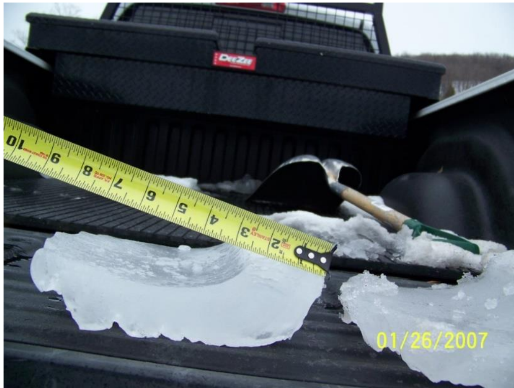
Figure 2.3 Ice fragment thrown from a wind turbine. Source: Munnsville Wind Farm, New York. Photo by Fred Gamlin.
