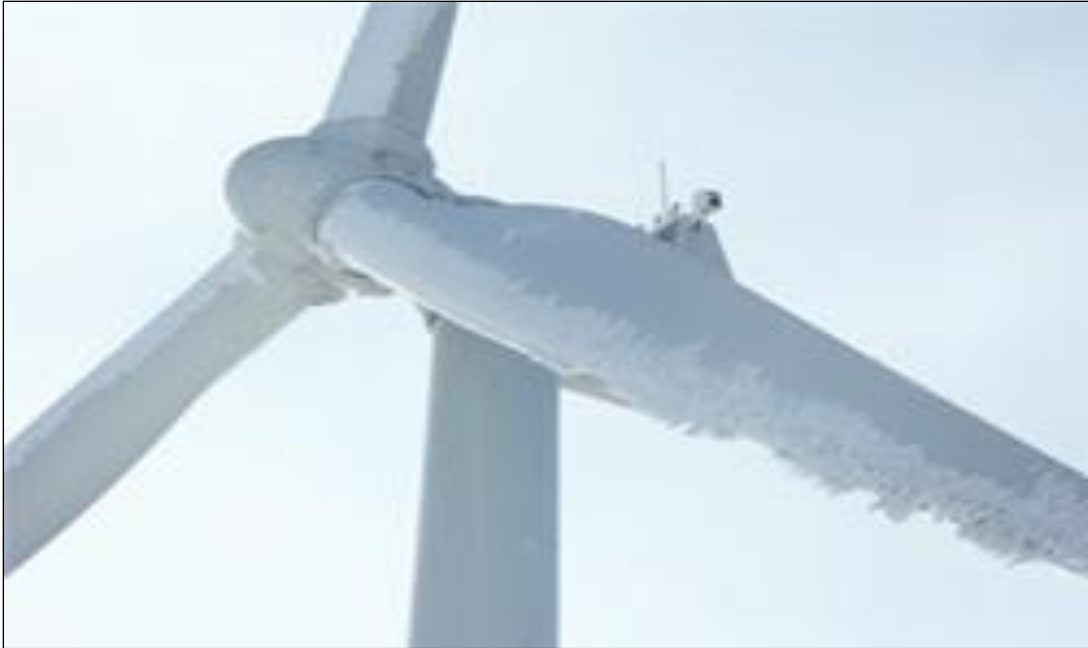
Figure 2.2 Ice forming on the leading edge of a wind turbine blade. Source: Wind turbine at Aapua-fjell, Sweden. Photo by Kent Larsson.
