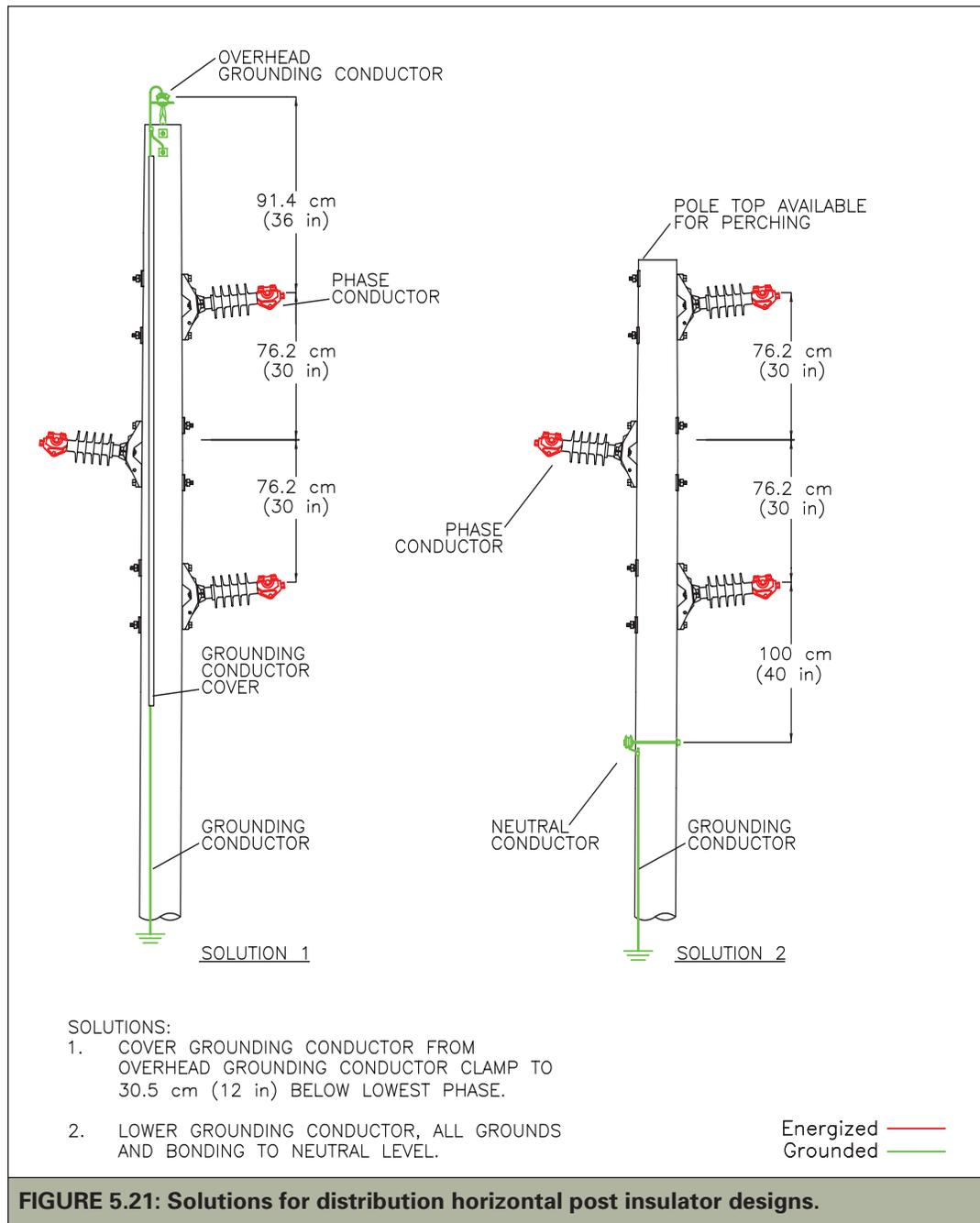
**FIGURE 5.21: Solutions for distribution horizontal post insulator designs.**
