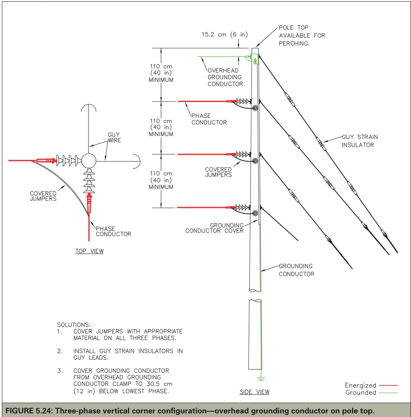
**FIGURE 5.24: Three-phase vertical corner configuration—overhead grounding conductor on pole top.**
