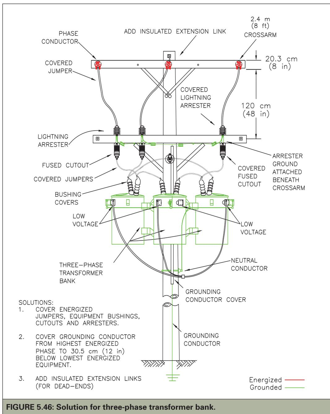
**FIGURE 5.46: Solution for three-phase transformer bank.**
