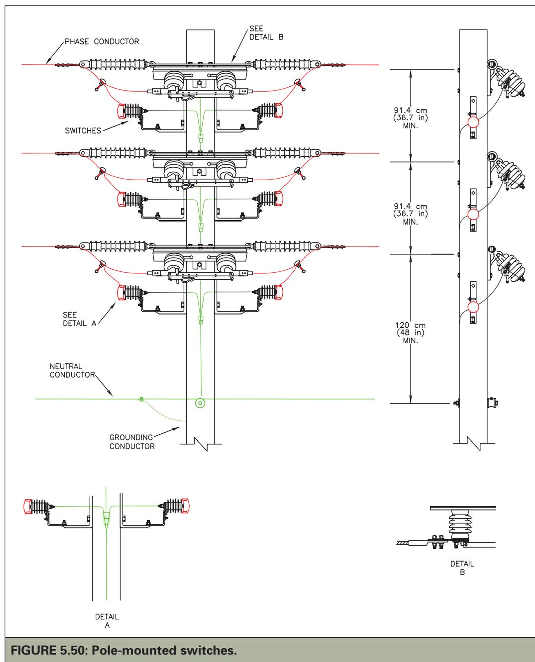
**FIGURE 5.50: Pole-mounted switches.**
