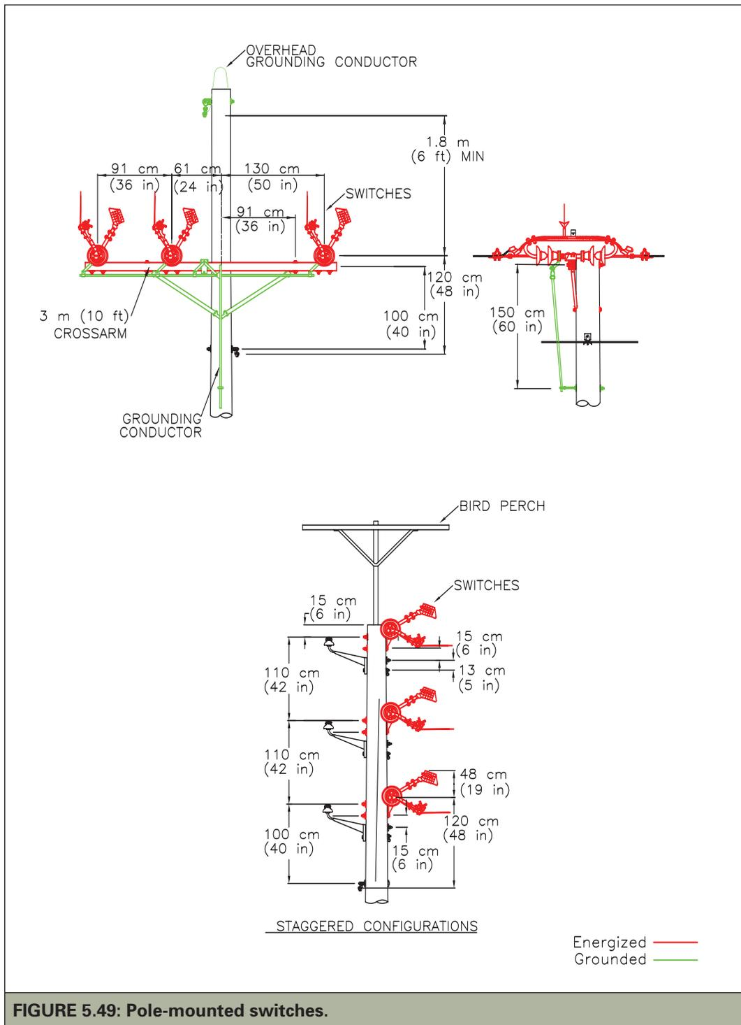
**FIGURE 5.49: Pole-mounted switches.**
