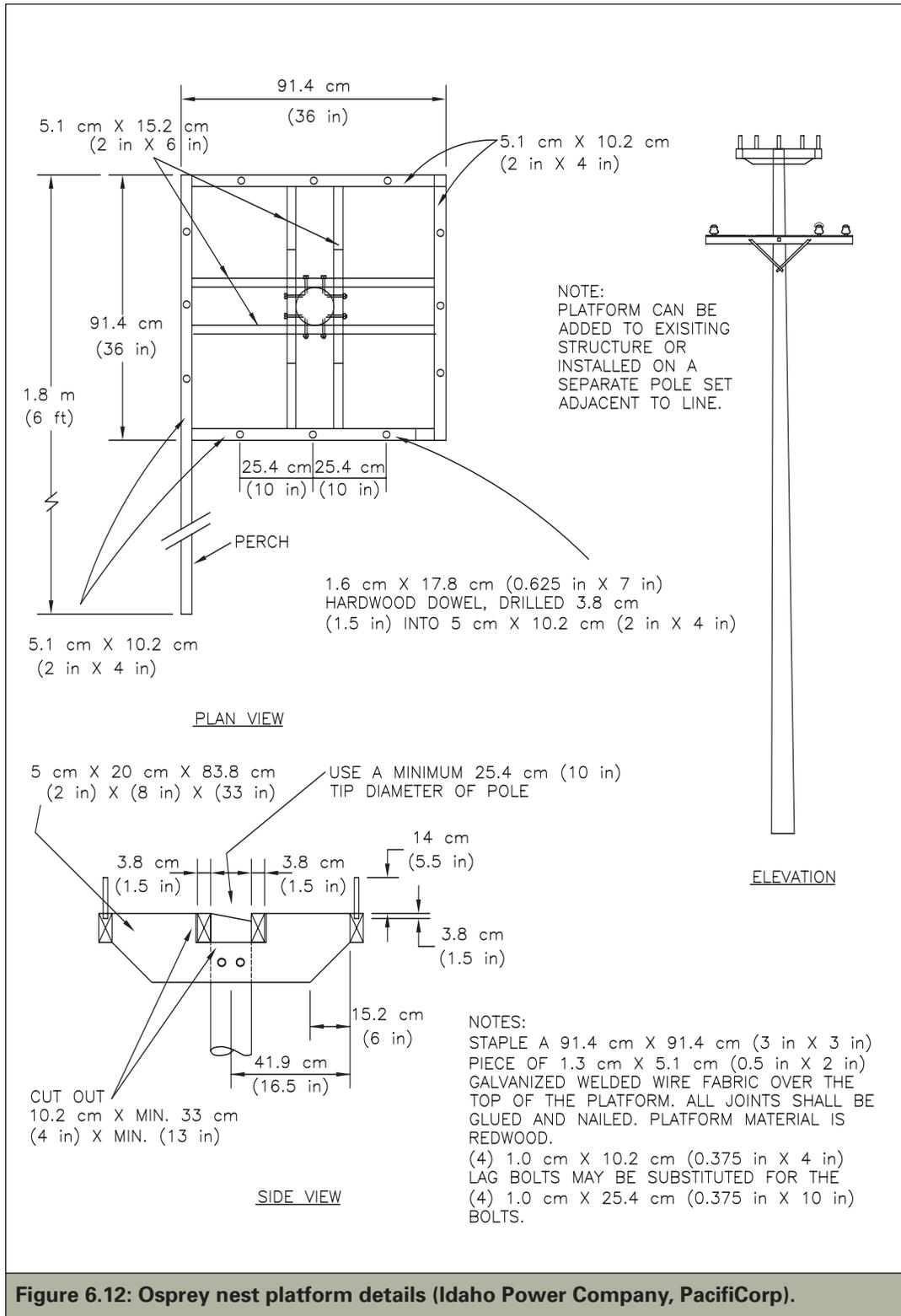
Figure 6.12: Osprey nest platform details (Idaho Power Company, PacifiCorp).
