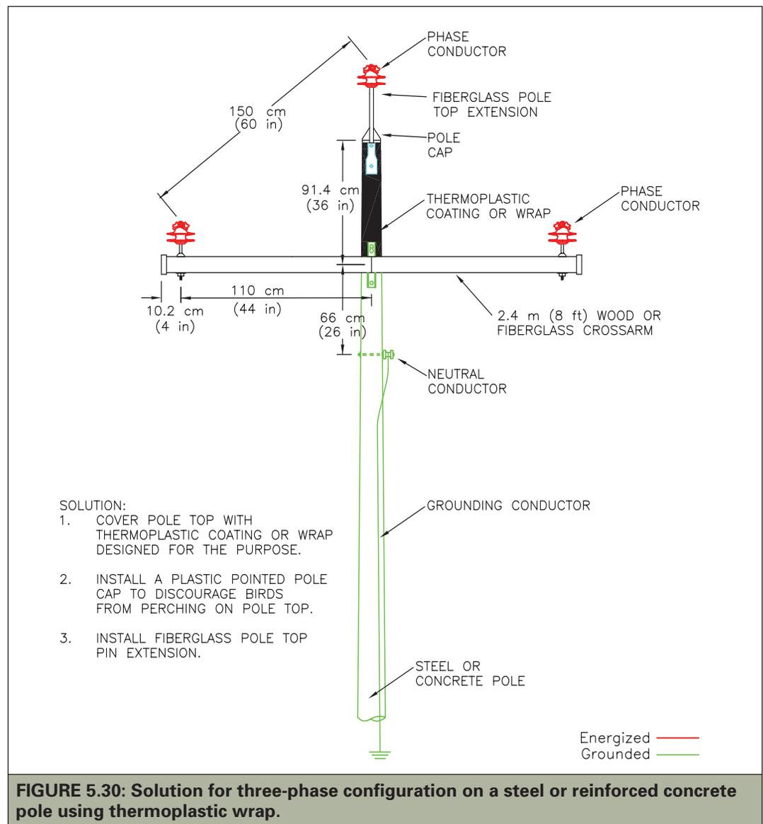
**FIGURE 5.30: Solution for three-phase configuration on a steel or reinforced concrete pole using thermoplastic wrap.**
