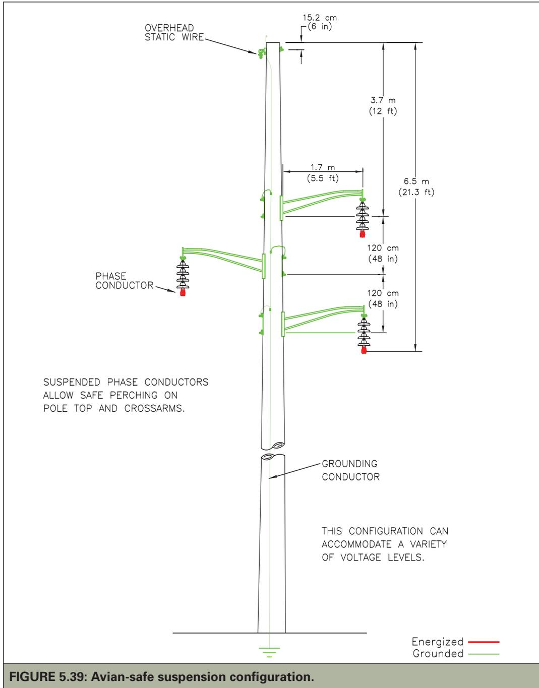
**FIGURE 5.39: Avian-safe suspension configuration.**
