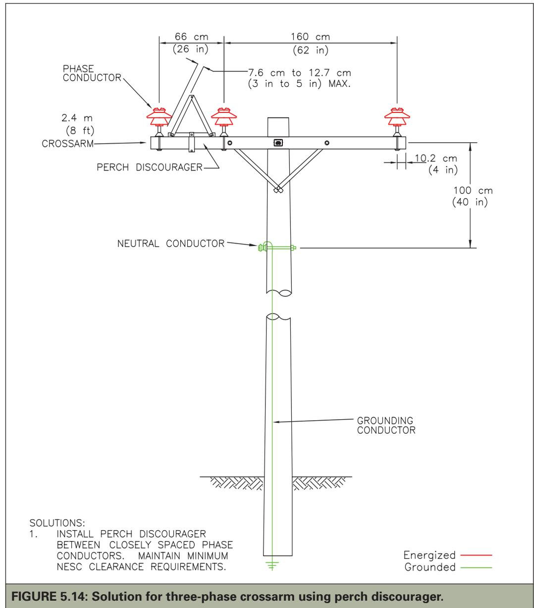
**FIGURE 5.14: Solution for three-phase crossarm using perch discourager.**
