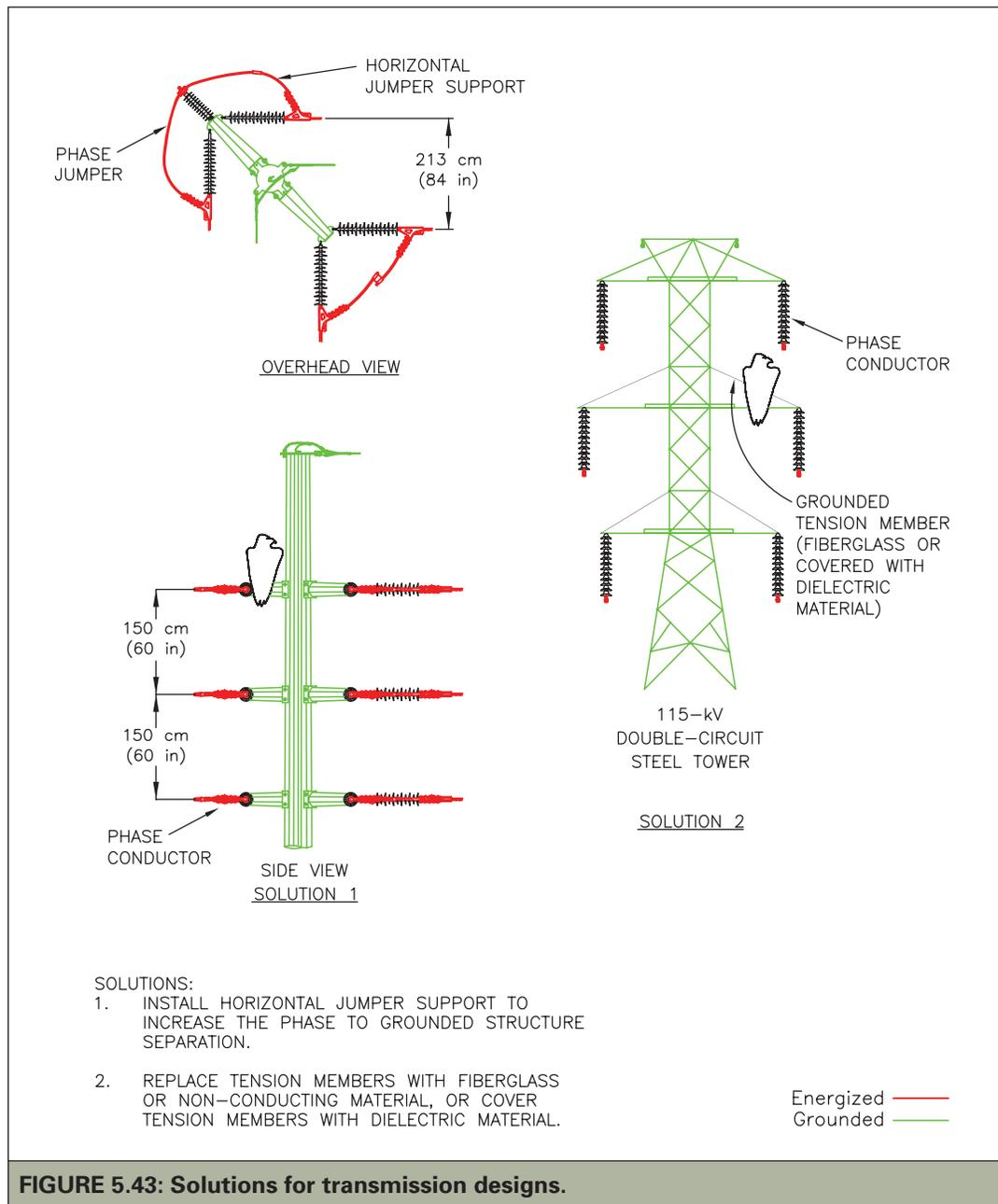
**FIGURE 5.43: Solutions for transmission designs.**
