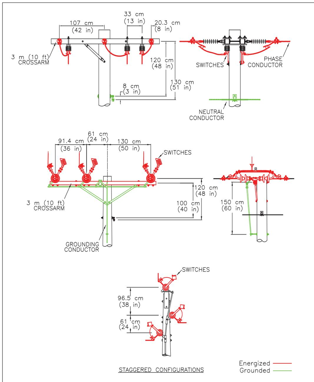
**FIGURE 5.48: Pole-mounted switches.**
