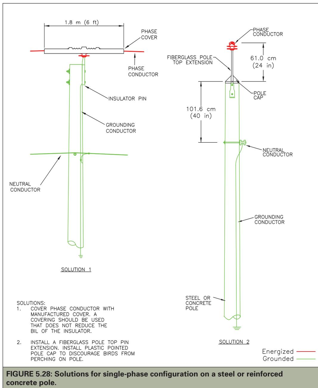
**FIGURE 5.28: Solutions for single-phase configuration on a steel or reinforced concrete pole.**
