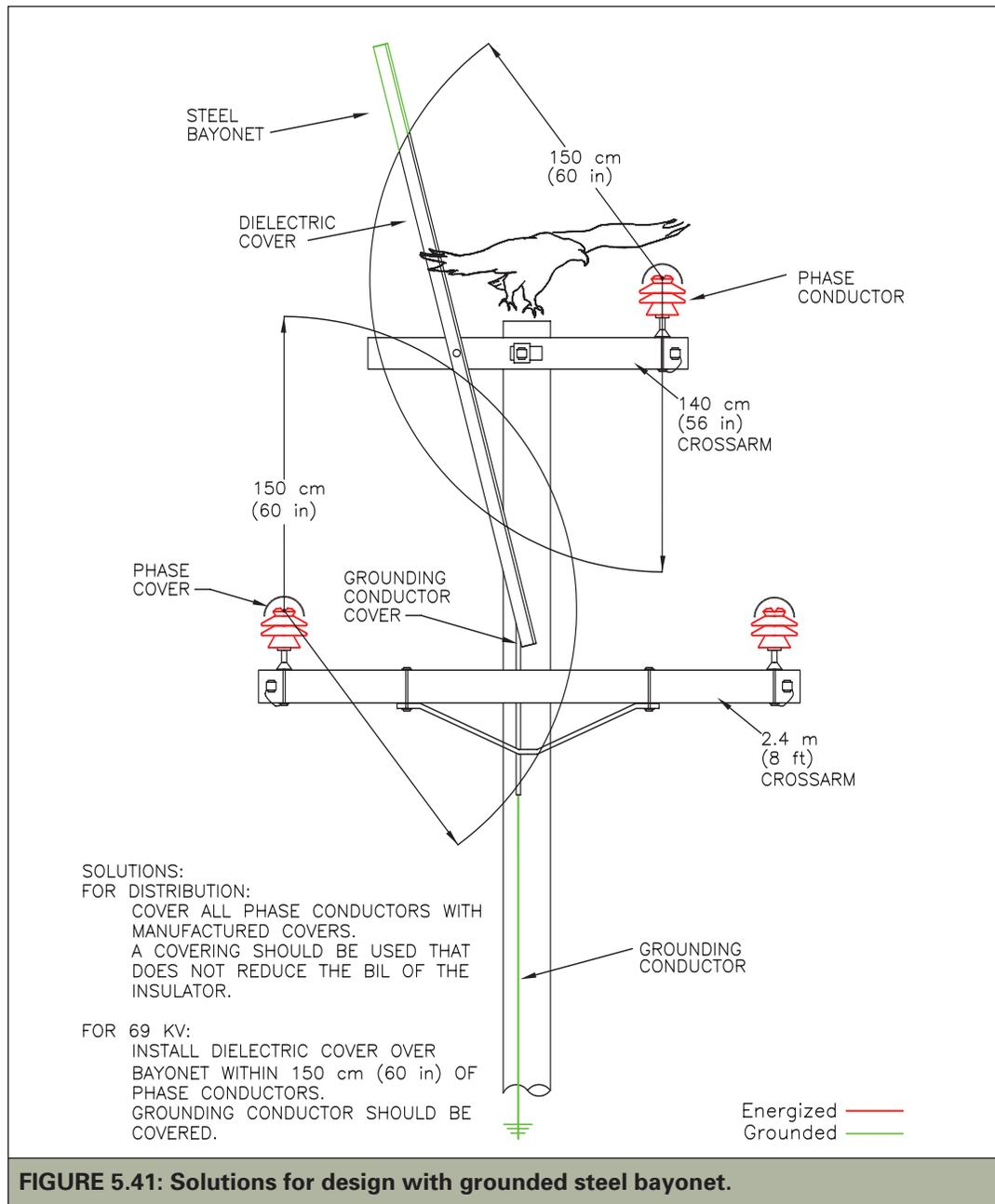
**FIGURE 5.41: Solutions for design with grounded steel bayonet.**
