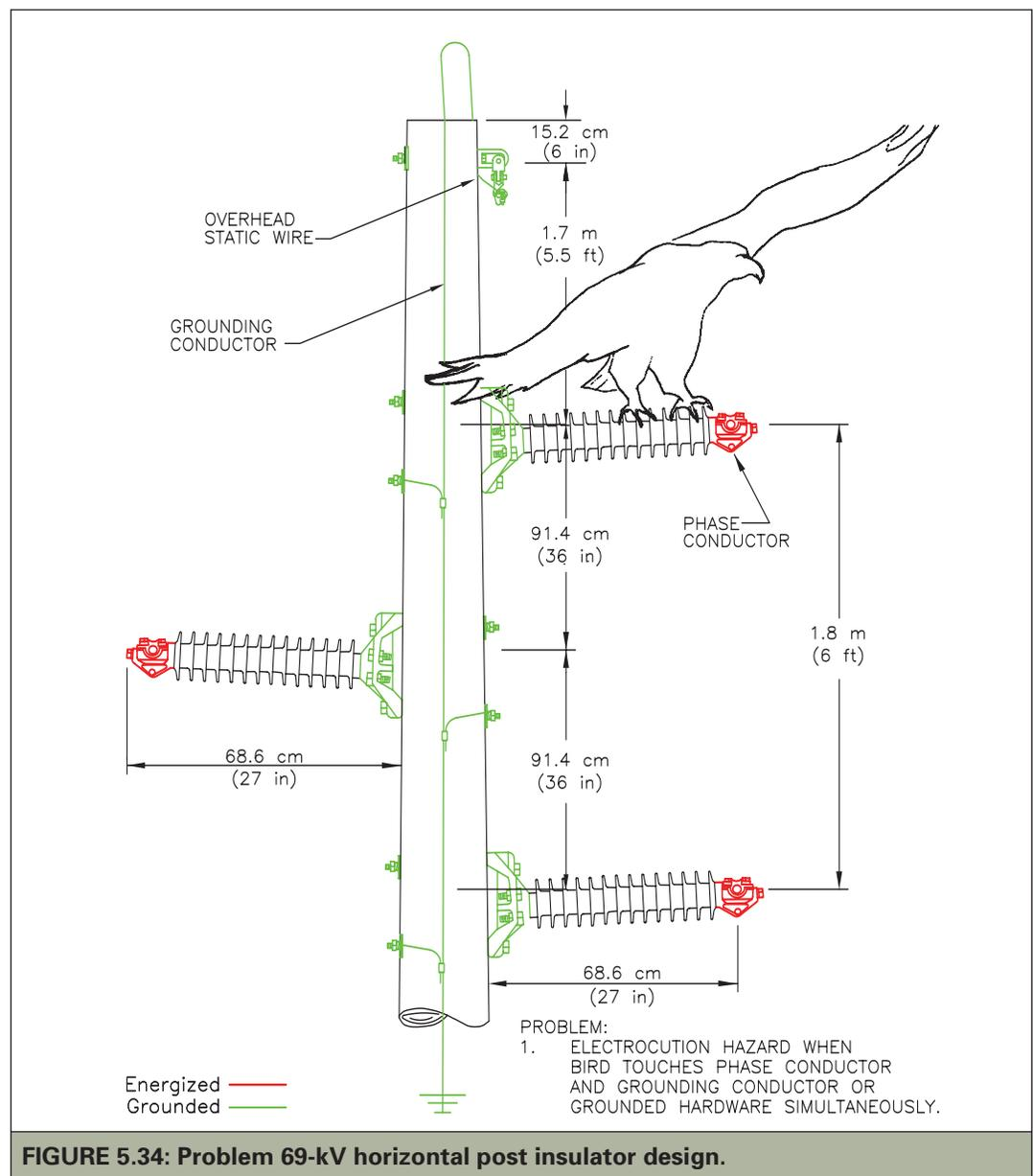
**FIGURE 5.34: Problem 69-kV horizontal post insulator design.**
