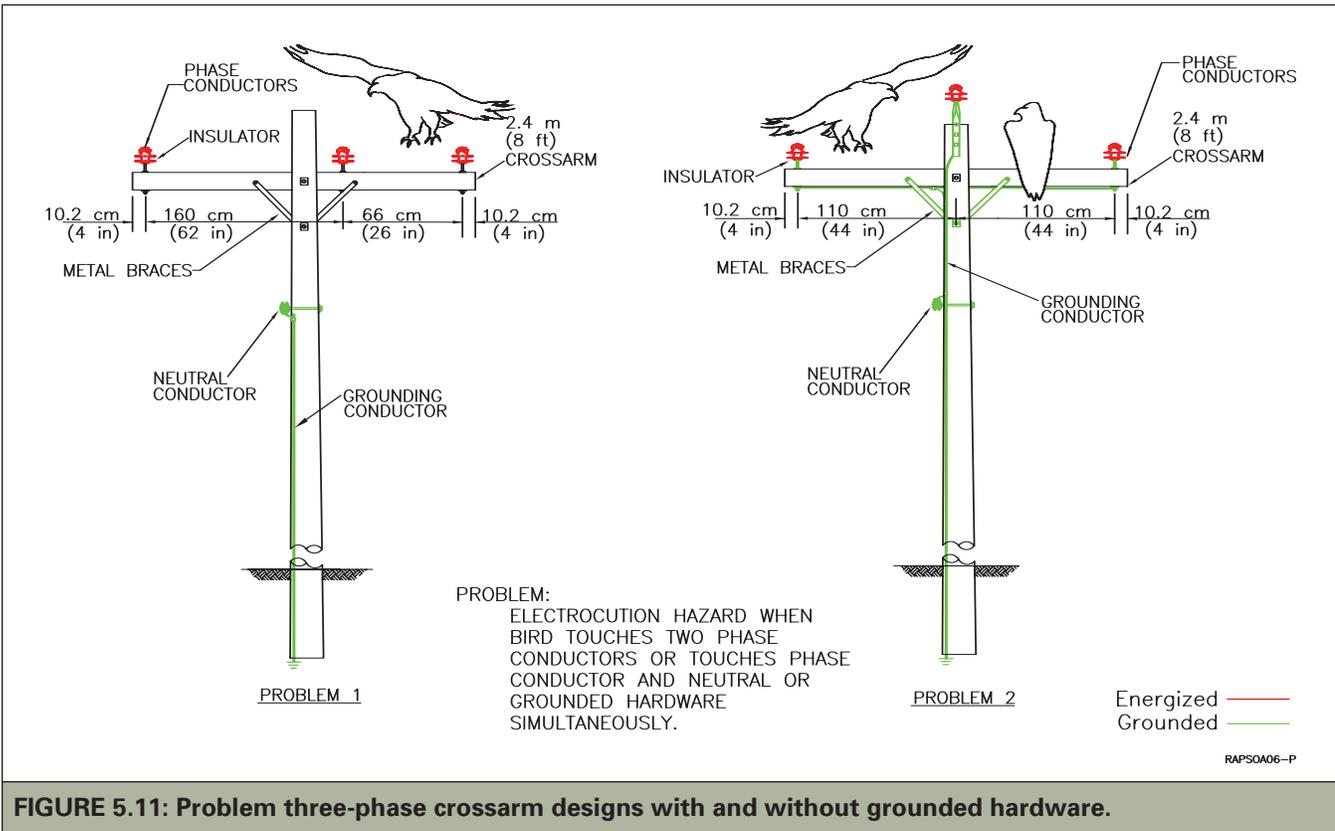
**FIGURE 5.11: Problem three-phase crossarm designs with and without grounded hardware.**
