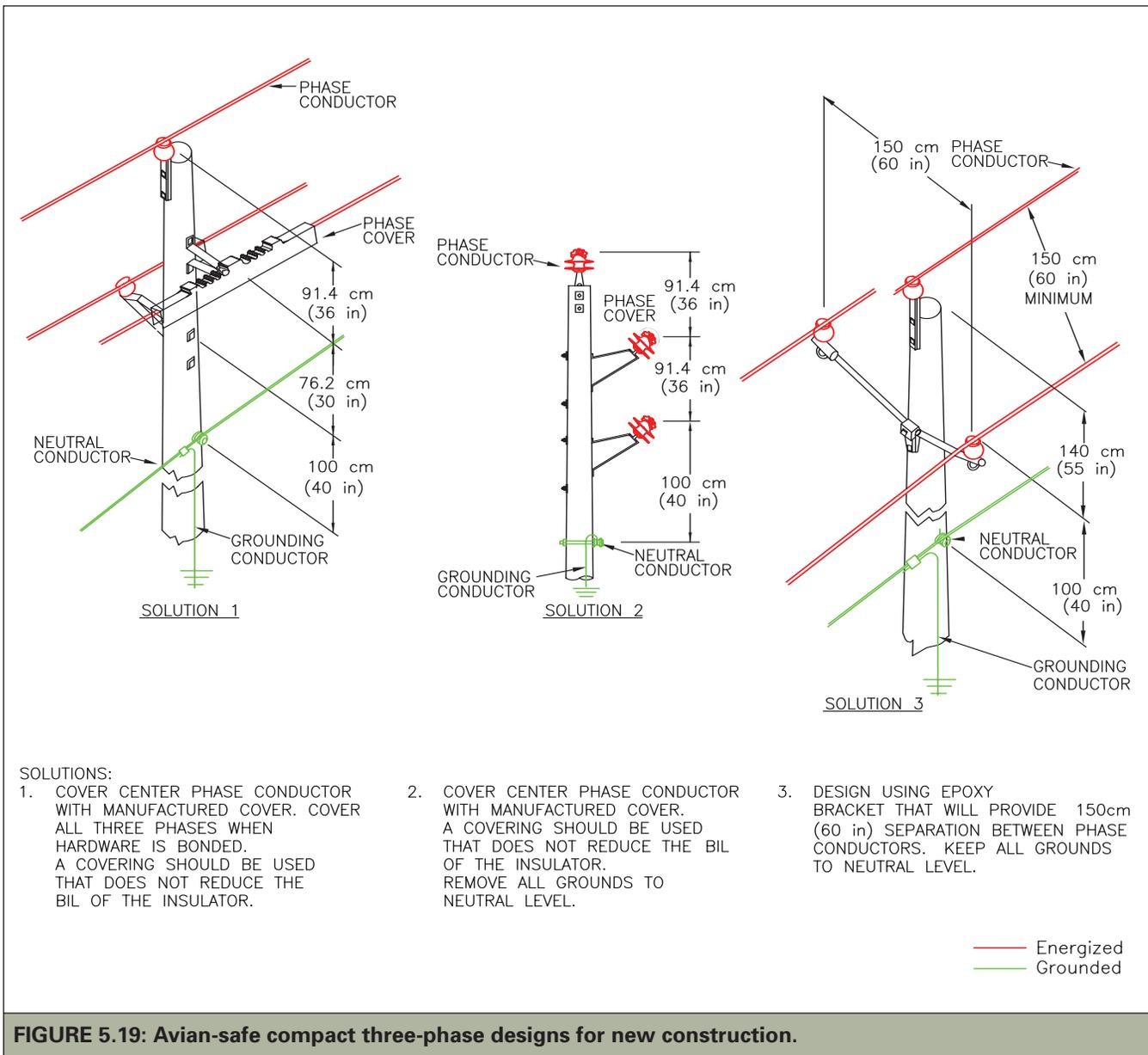
**FIGURE 5.19: Avian-safe compact three-phase designs for new construction.**
