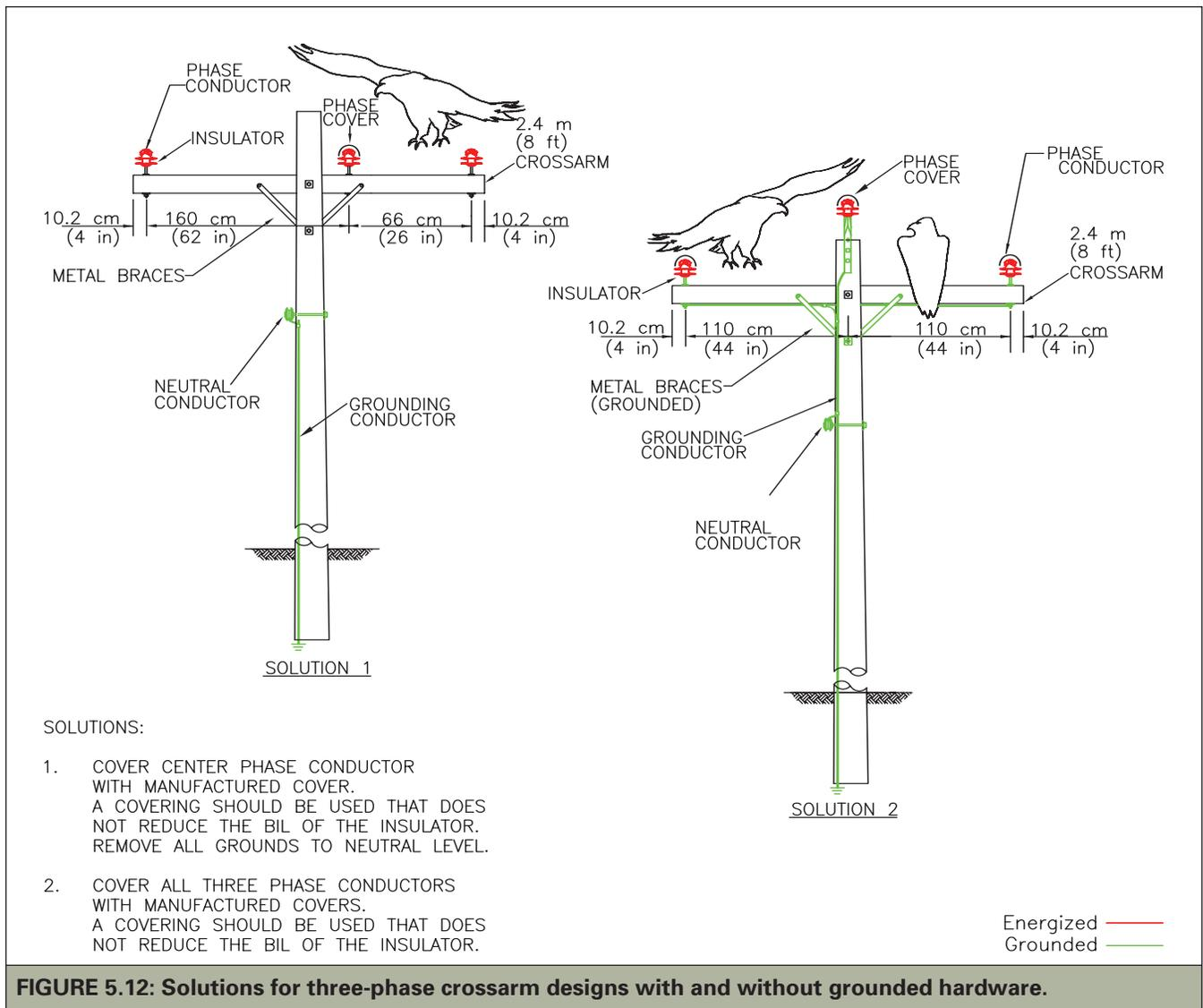
**FIGURE 5.12: Solutions for three-phase crossarm designs with and without grounded hardware.**
