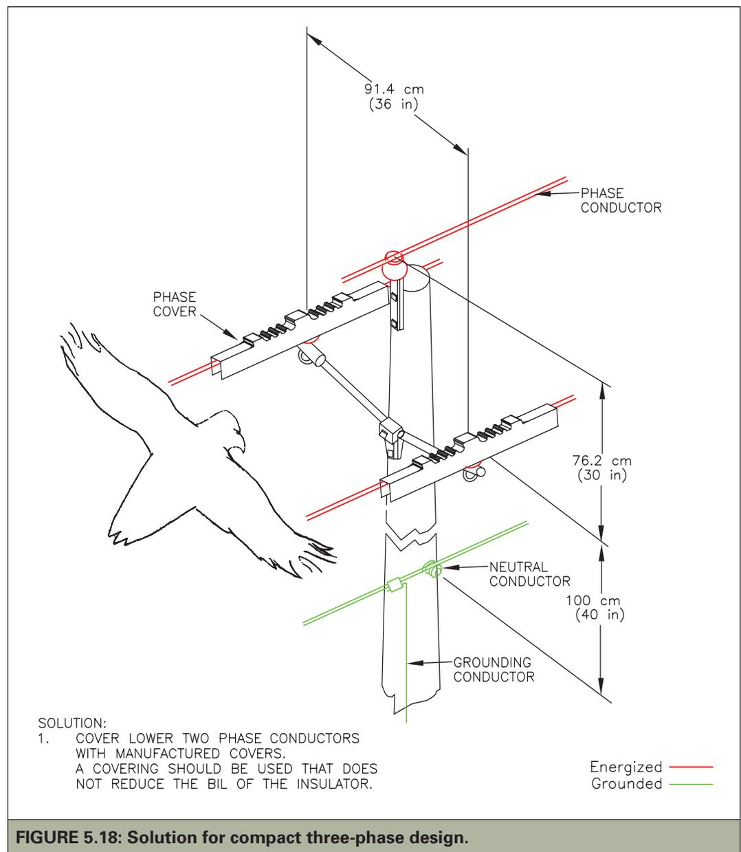
**FIGURE 5.18: Solution for compact three-phase design.**
