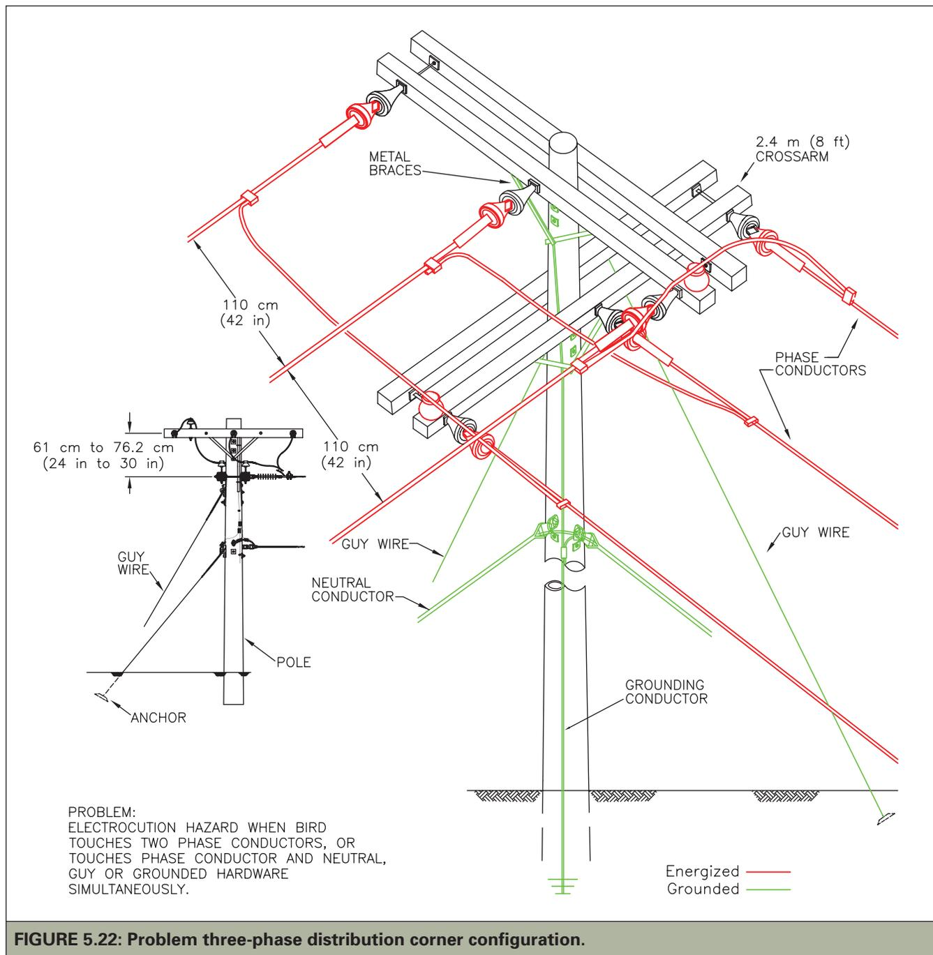
**FIGURE 5.22: Problem three-phase distribution corner configuration.**
