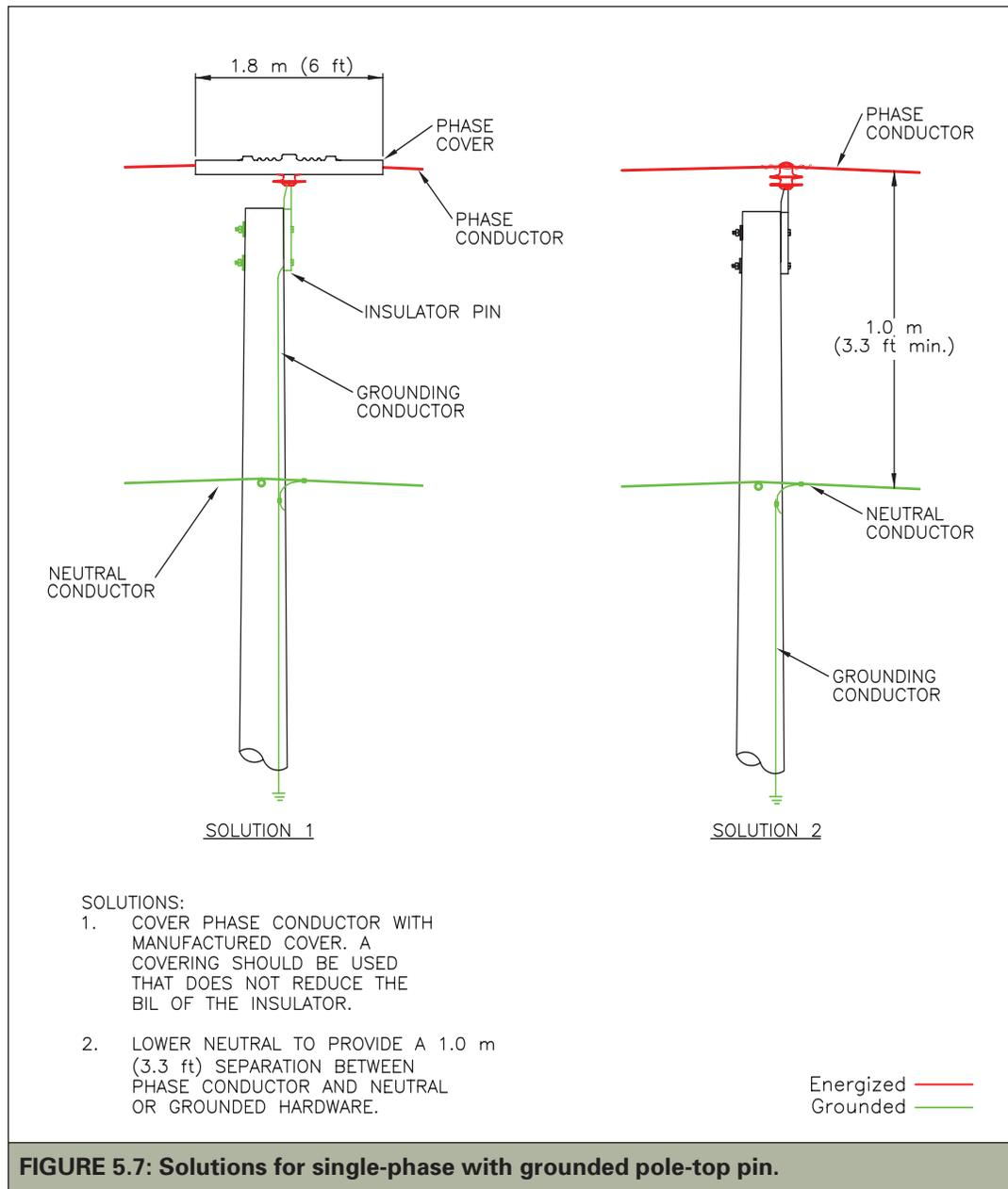
**FIGURE 5.7: Solutions for single-phase with grounded pole-top pin.**
