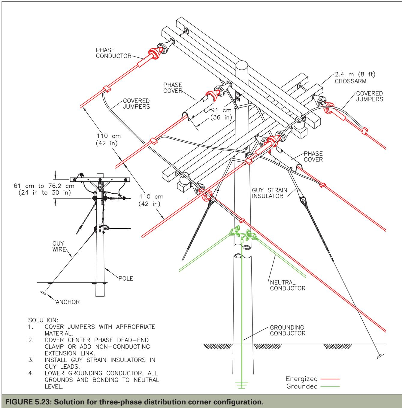
**FIGURE 5.23: Solution for three-phase distribution corner configuration.**
