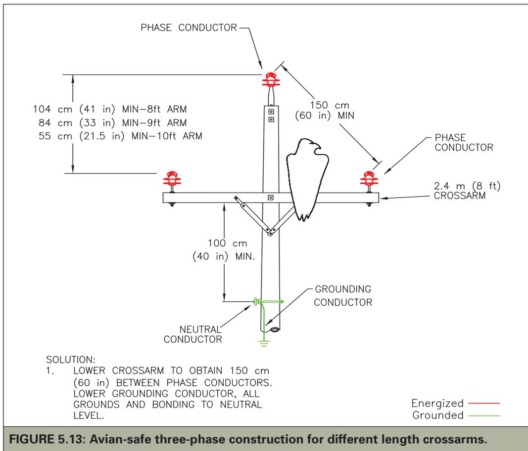
**FIGURE 5.13: Avian-safe three-phase construction for different length crossarms.**
