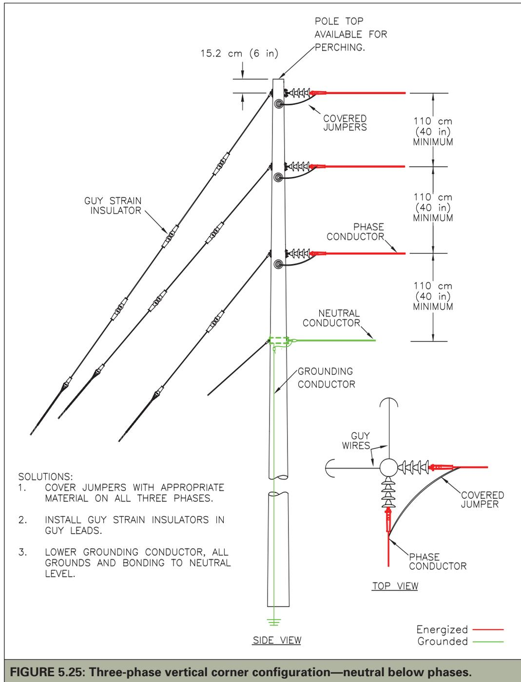
**FIGURE 5.25: Three-phase vertical corner configuration—neutral below phases.**
