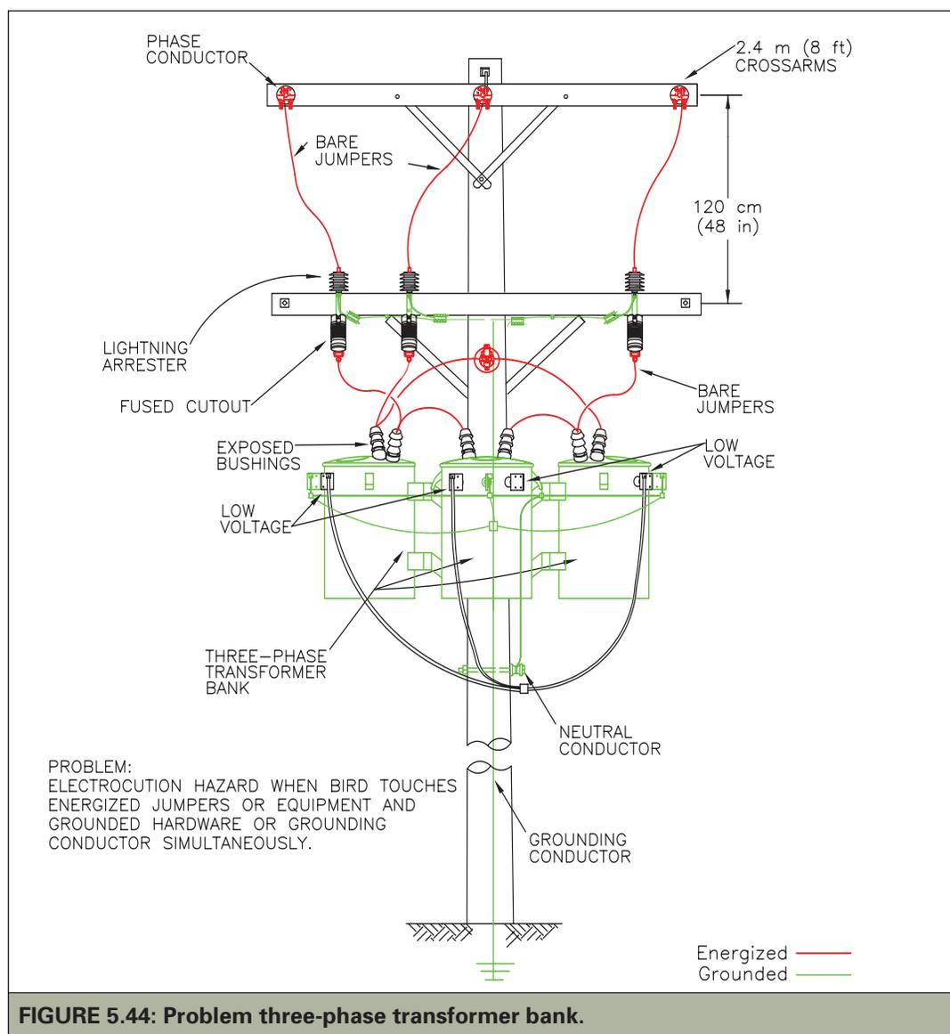
**FIGURE 5.44: Problem three-phase transformer bank.**
