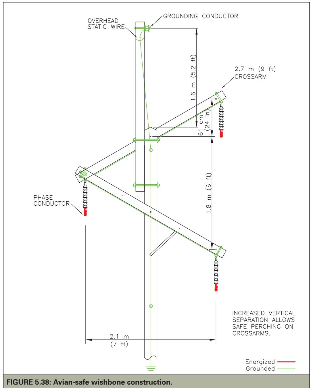
**FIGURE 5.38: Avian-safe wishbone construction.**
