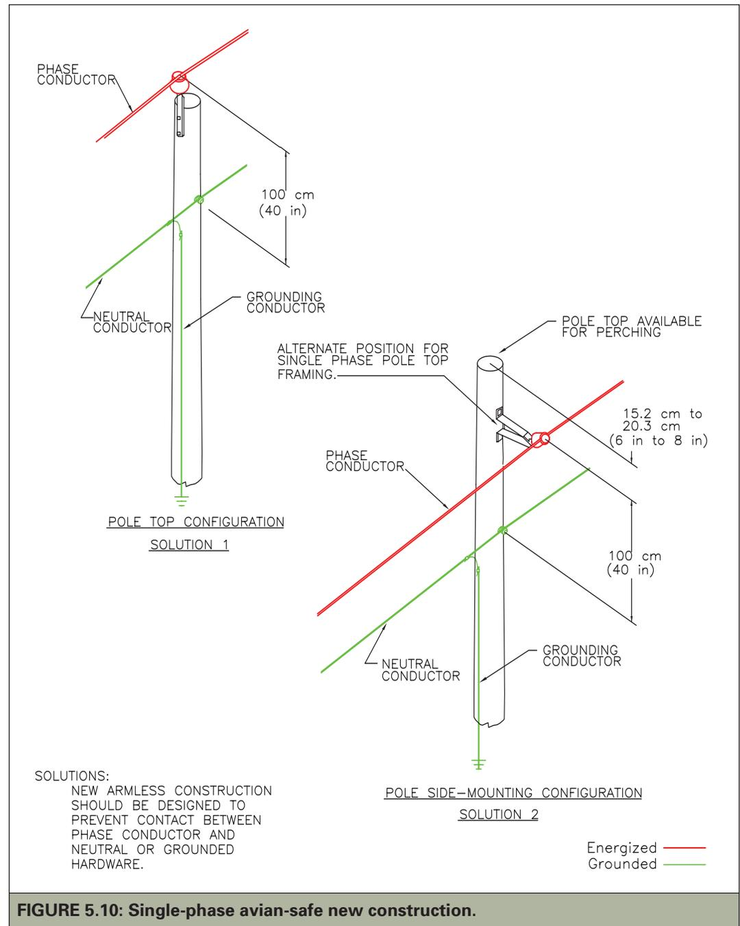
**FIGURE 5.10: Single-phase avian-safe new construction.**
