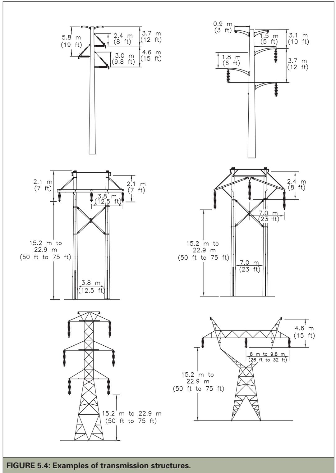
**FIGURE 5.4: Examples of transmission structures.**
