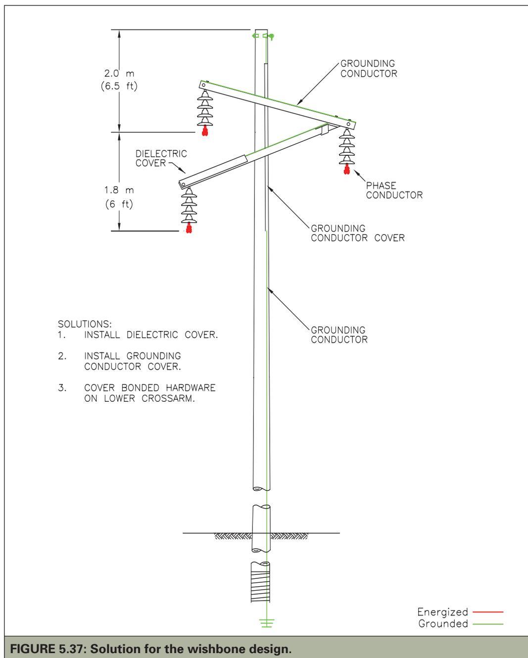
**FIGURE 5.37: Solution for the wishbone design.**
