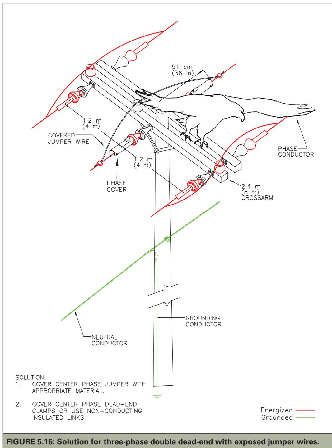
**FIGURE 5.16: Solution for three-phase double dead-end with exposed jumper wires.**
