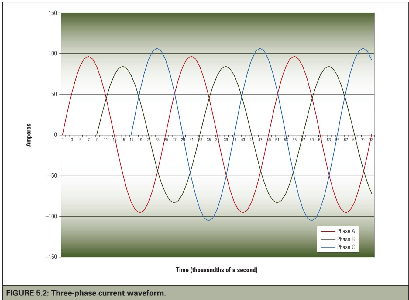
**FIGURE 5.2: Three-phase current waveform.**
