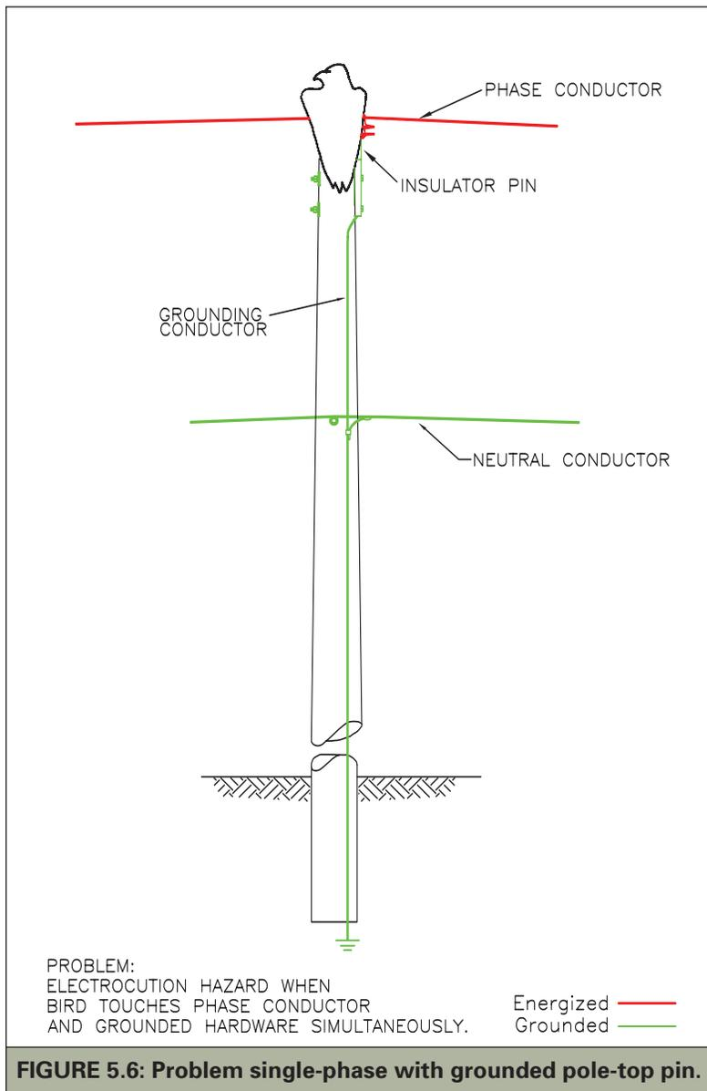
**FIGURE 5.6: Problem single-phase with grounded pole-top pin.**
