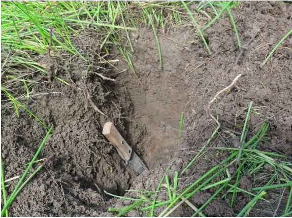
Photo 1. View of soil pit at Sample Site 8 that showed evidence of depletions and redoximorphic concentrations. 04/16/2019
