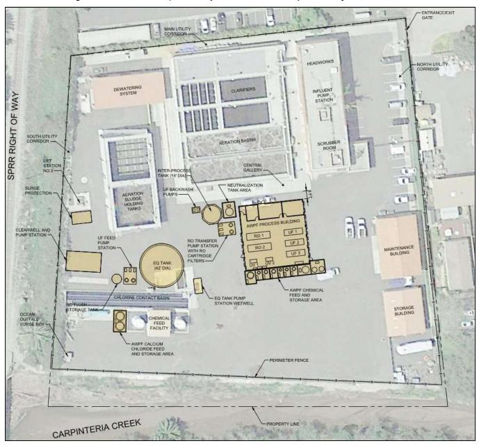
Figure Error! No text of specified style in document.: Proposed Project Site Plan at CSD WWTP
