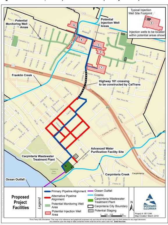
Figure Error! No text of specified style in document.: Conceptual Layout of Proposed Facilities
