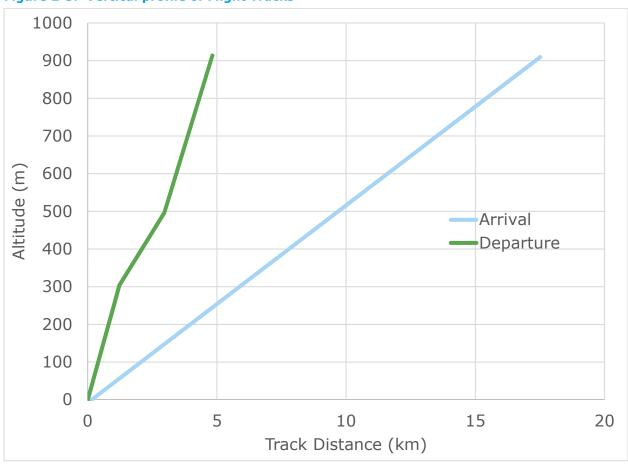
Figure 2-3. Vertical profile of Flight Tracks
