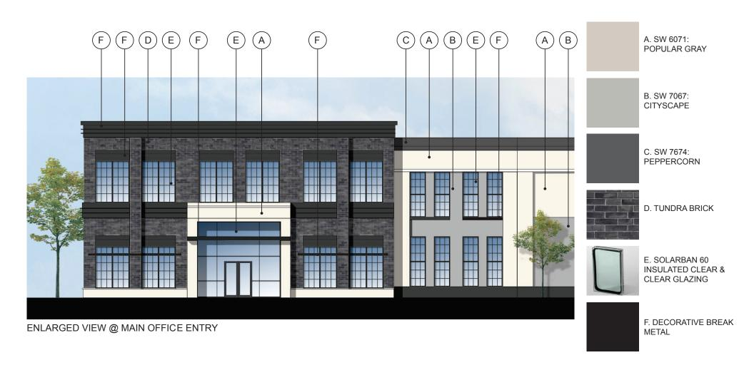
Figure 3-10a Proposed Materials for the Main Building Entry at Southeast Corner
