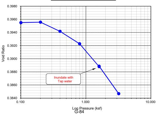
Void Ratio - Log Pressure Curve
