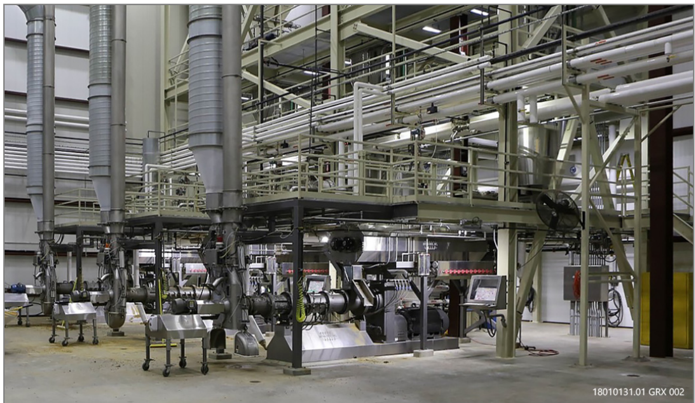
Figure 2-3 Existing Three Lines (Steam Conditioners) with Space for Fourth Conditioner
