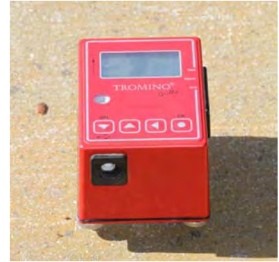
Tromino ENGR used for HVSR measurements in shallow basins
