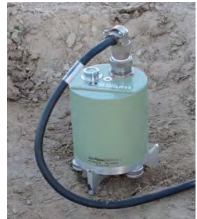
Trillium Compact 120 second seismometer used for HVSR measurements in deep basins
