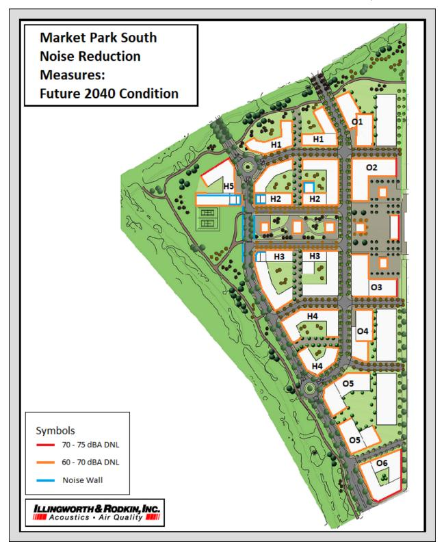
FIGURE 3 Noise Reduction Measures Needed for General Plan Consistency
