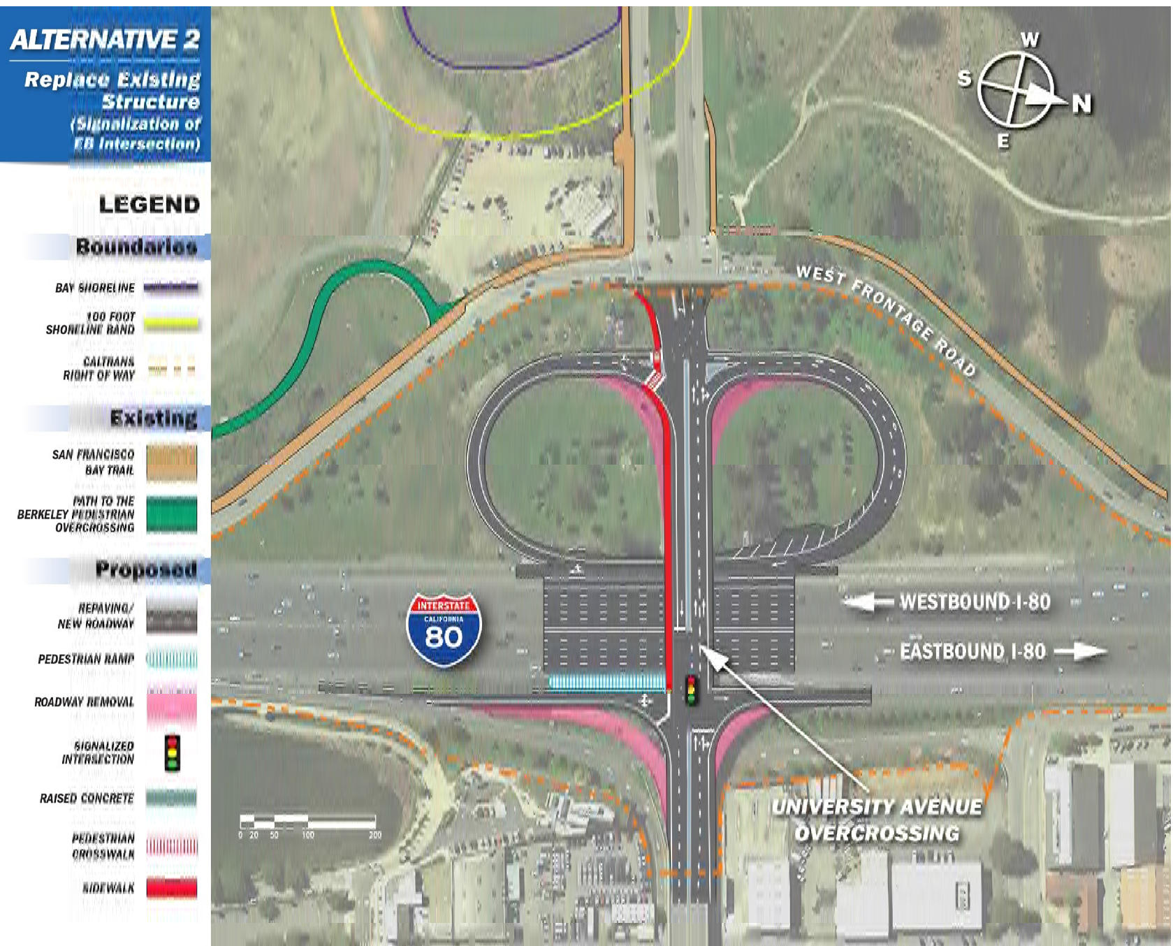
Figure 1-3: Alternative 2, Replace Existing Structure (Signalization of EB Intersection)
