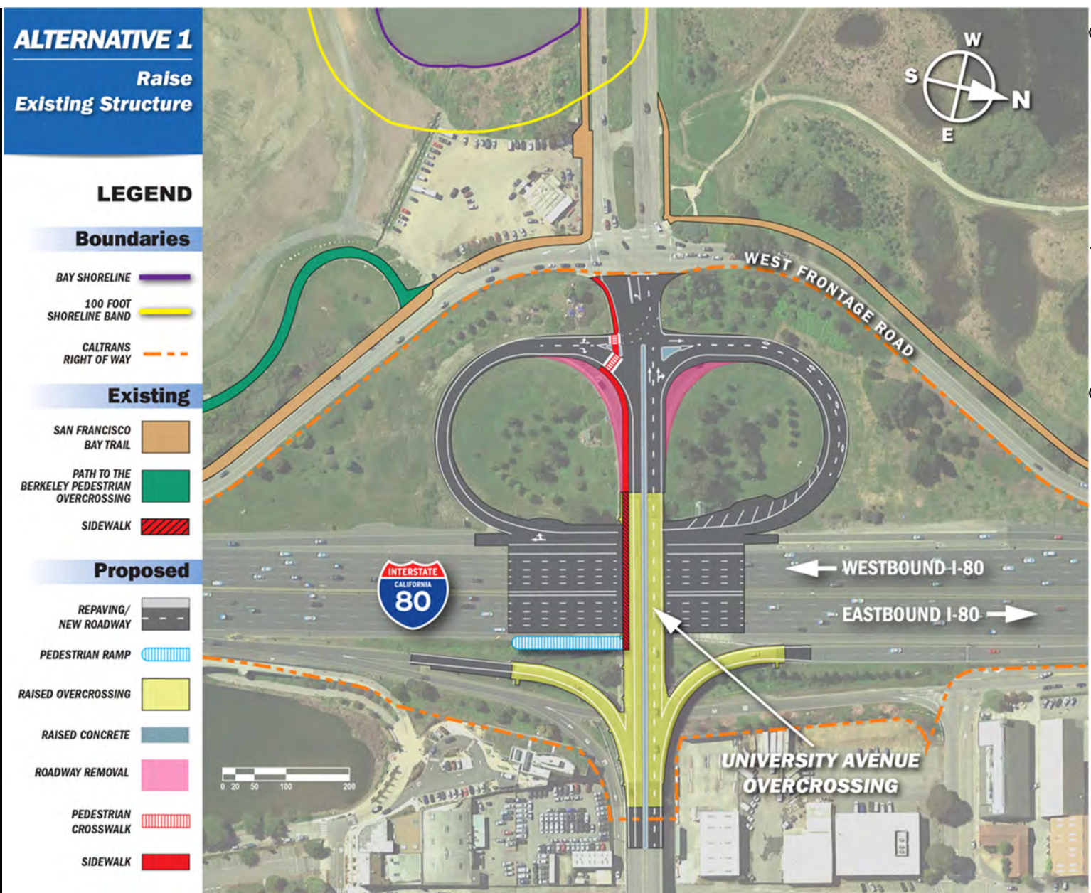
Figure 1-2: Alternative 1, Raise Existing Structure
