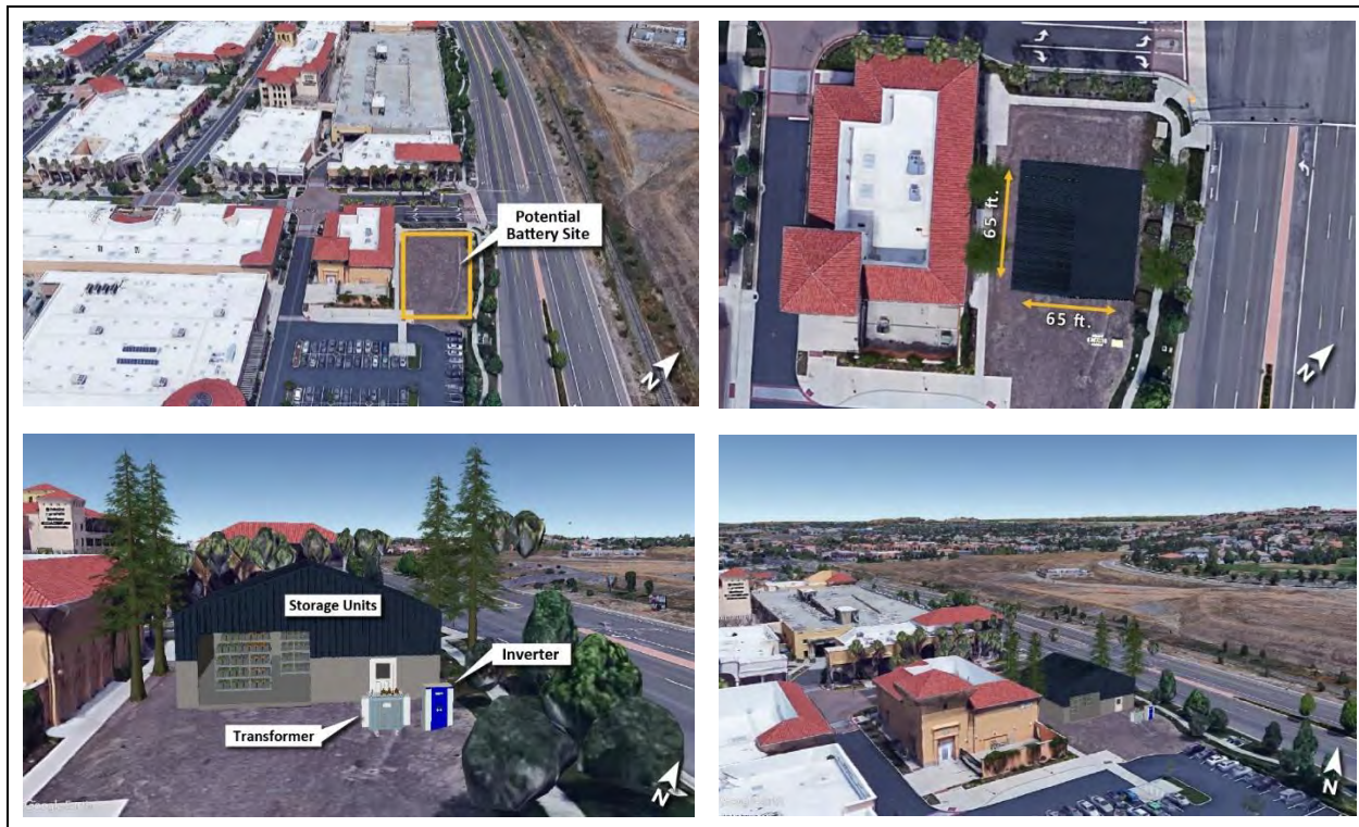
Figure 3-25. Example Energy Storage Facility Enclosed in Building
