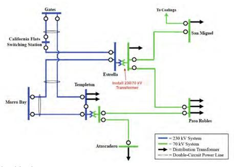
Figure 2-3. Proposed Transmission System – Line Diagram
