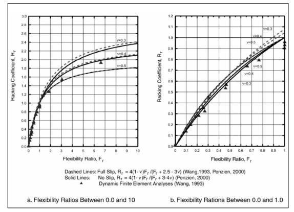
Figure 3B-9 Racking Ratio Coefficient R<sub>r</sub> for Rectangular Box Structures (MCEER-06-SP11, Modified from Wang, 1993, and Penzien, 2000)
