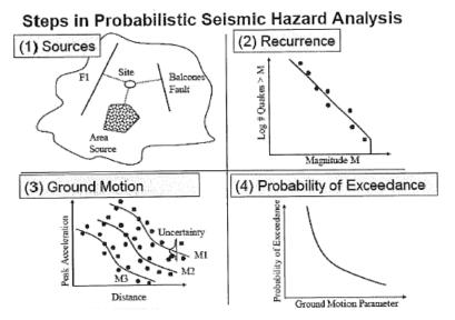
Figure 2-4 Steps in Probabilistic Seismic Hazard Analysis
