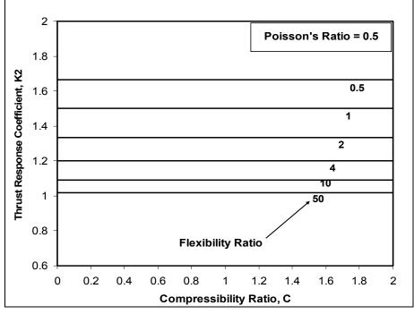
Figure 3B-6 Lining Response Coefficient, K<sub>2</sub>, for Poisson's Ratio = 0.5 (Wang, 1993)
