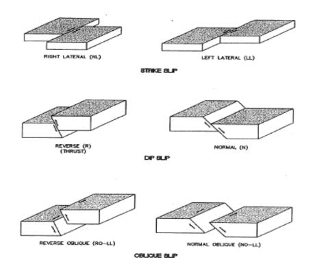
Figure 2-7 Types of earthquake faults
