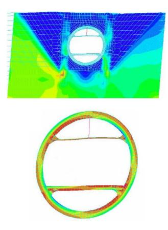
Figure 3B-7 Example of Two-dimensional Continuum Finite Element Model
