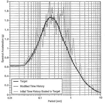
Figure 2-5 Example of Acceleration Spectral Matching
