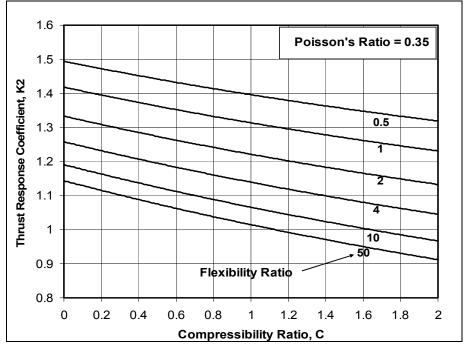
Figure 3B-5 Lining Response Coefficient, K<sub>2</sub>, for Poisson's Ratio = 0.35 (Wang, 1993)
