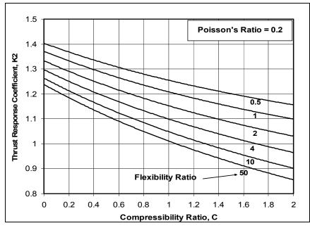
Figure 3B-4 Lining Response Coefficient, K<sub>2</sub>, for Poisson's Ratio = 0.2 (Wang, 1993)
