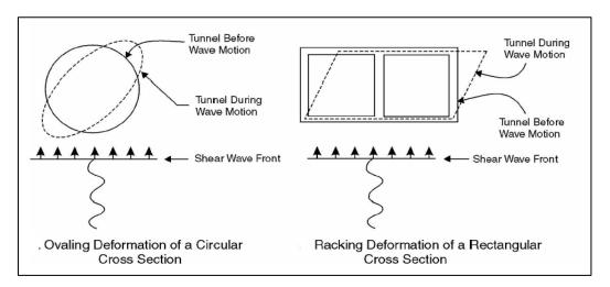
Figure 3B-1 Tunnel Transverse Ovaling and Racking Response to Vertically Propagating Shear Waves (Wang, 1993)
