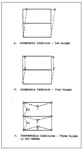
Figure 3B-12 Structure Mechanisms under MDE
