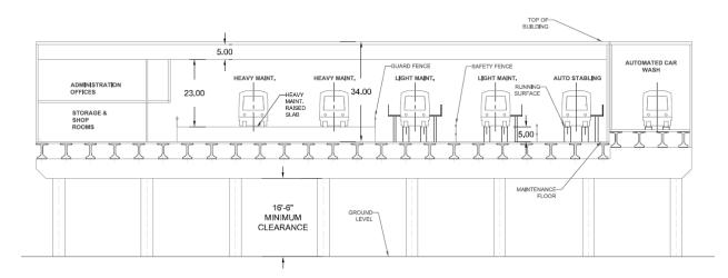
Figure 8-9: MSF Cross Section
