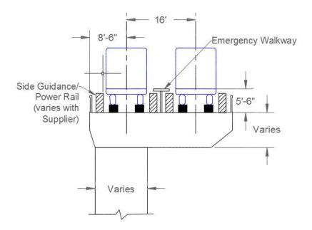
Figure 7-1: APM Guideway Clearances - Dual Track
