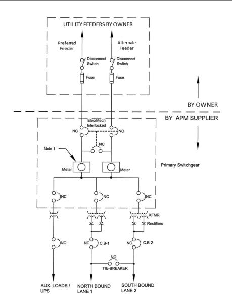
Figure 9-2: Typical Single Line Diagram
