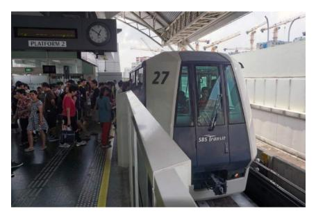
Figure 6-1: Singapore Sengkang LRT Station with Half-height Barrier Wall/Platform Doors, MHI Crystal Mover APM (Image Credit: Peter Velthoen)
