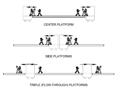
Figure 6-2: Profile views of Platform Configurations
