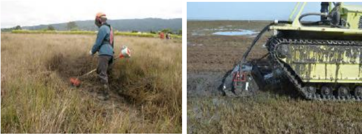
Image 2-1 – Representative Vegetation Removal Equipment. Handheld brushcutter (left) used to remove above-ground vegetation. Marshmaster (right) used to mow larger areas and grind (via rototiller) dense-flowered cordgrass rhizomes. Photo credit: A. Pickart (USFWS 2017)
