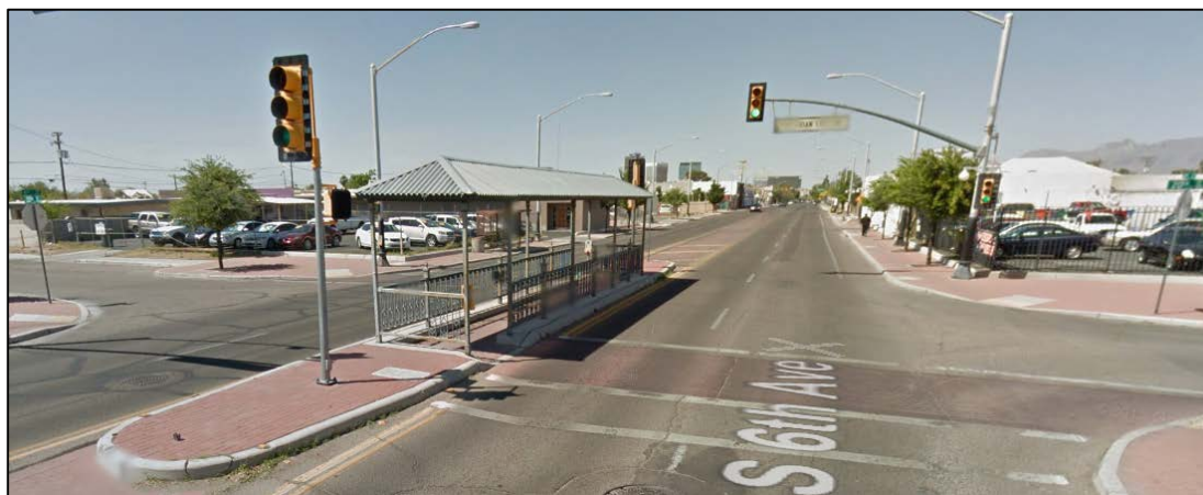
Figure 6-50: Two-stage Pelican crossing in Tucson, AZ
