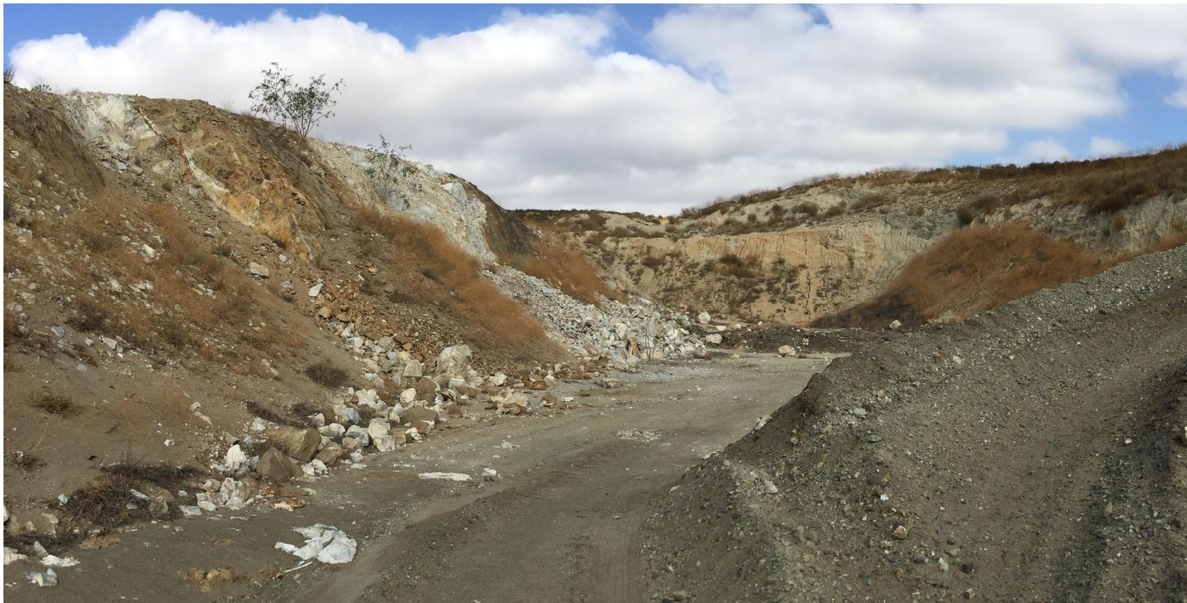
Photo 9: Location 3 – Shallow quarry in marble (white) bounded by metasediments (schist).
