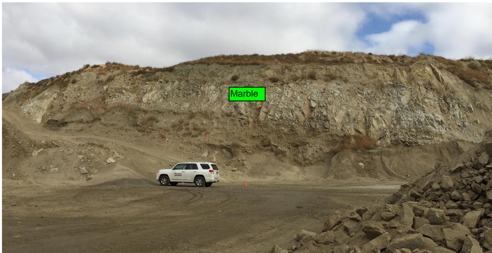
Photo 8: Location 2 – north cut. Marble bed dipping away from viewer.
