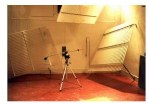
Figure 12. Barrier absorption: Reverberation Room Method photo #2553
