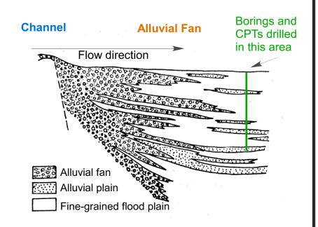
Longitudinal Profile of an Alluvial Fan and Alluvial Plain showing the flattening of the geologic units in the distal portion of the fan, in the approximate area where Sections M-M' and N-N' are located. Alluvial fan diagram modified from Fraser and Suttner (1986).
