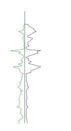
CPT Log. Blue line is Cone Resistance (qc in tsf). Green line is Sleeve Friction (fs in tsf).
