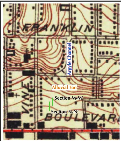
Location of Sections M-M' and N-N' relative to the Argyle Fan. Note that the sections are somewhat oblique to gradient of the fan. Base map is c. 1926 topography from Hoots and Kew (1931).
