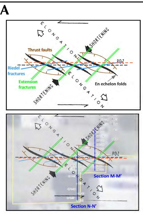
A (above): Orientation of en echelon folds and faults in left simple shear, such as those anticipated along the left-lateral Hollywood fault. PDZ = principal displacement zone. (Modified from Sylvester, 1988). Bottom diagram shows how these features would project across a section of the East Millennium site assuming that the southern feature in Section M-M' is real, and part of a left-lateral zone of slip with a predominantly east-towest strike.
