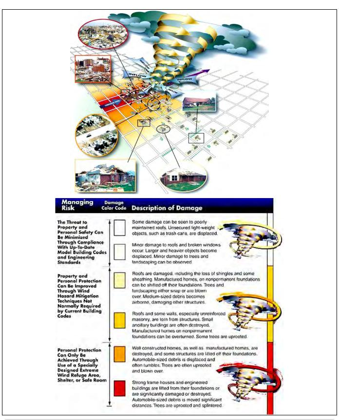
Figure 6-1. Potential Impact and Damage from a Tornado
