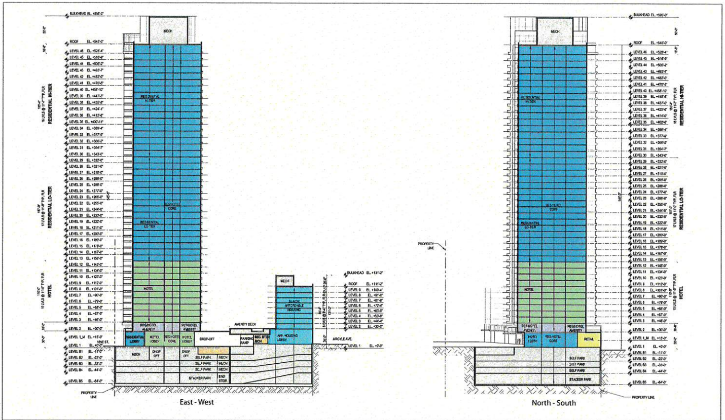
Figure 5 Hotel Option Building Sections, East Site
