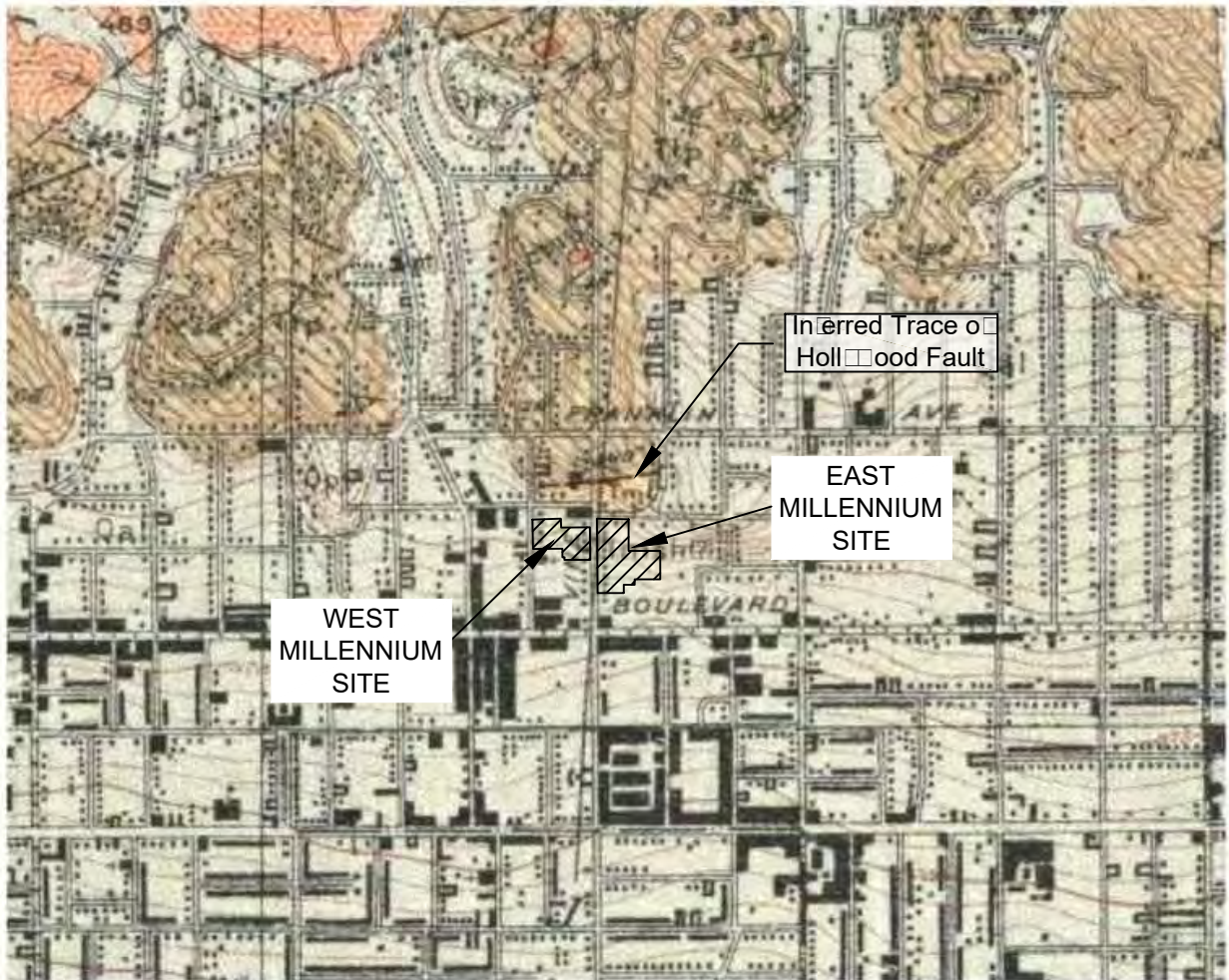
Figure 3: Geologic map of Millennium site and vicinity (after Hoots and Kew, 1931) showing inferred trace of a Hollywood Fault separating Modelo ( T_m ), and Topanga ( T_t ) Formations, granite rocks (gr), and alluvium ( Q_{al} ).
