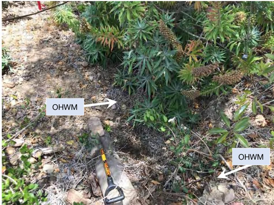
Photo 11. Upstream view of F1 showing the WSP 5 soil sample pit. Wetland hydrology parameter met; dominant or prevalent hydrophytic vegetation and hydric soils not present.
