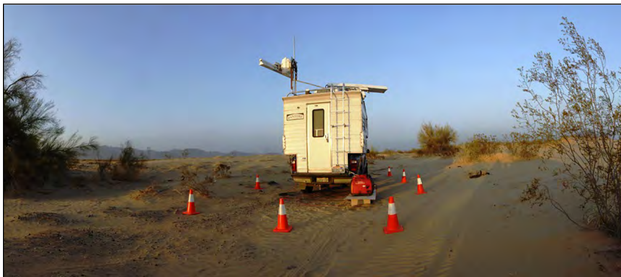
Figure 3. Furuno Model FR-1510 Mark 3 modified marine radar units utilized for nocturnal radar sampling, as mounted on a pickup truck camper.
