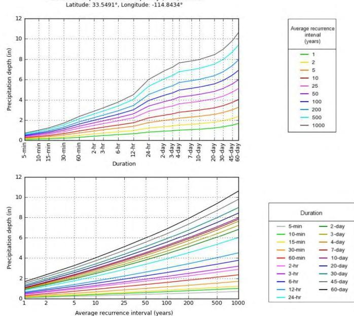
PDS-based depth-duration-frequency (DDF) curves Latitude: 33.5491°, Longitude: -114.8434°
