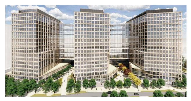
Figure 3. View of the south façade of the CityView Plaza building. Fins and mullions break up the facades of the towers and make the building more visible to birds. However, the transparent glass bridges are a collision hazard because birds can see through to the other side of the bridge, and will collide with the glass when they attempt to fly through to the far side of the bridge.
